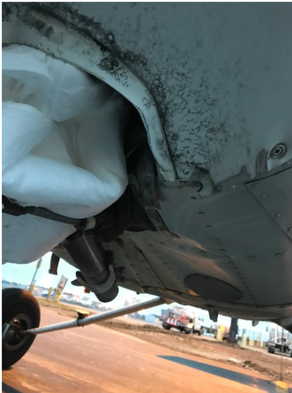
Photo 2 – View of damaged fuselage from underneath (Photo courtesy of the FAA)
