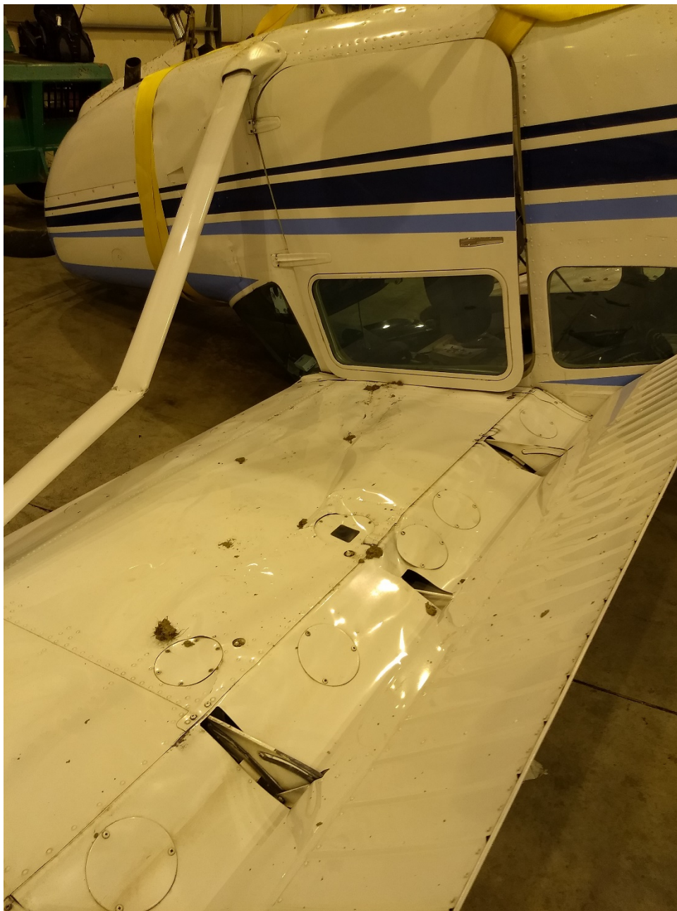
Photo 2 – View of right wing and lift strut damage (Photo courtesy of the FAA)
