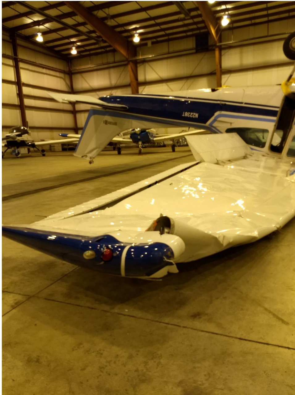
Photo 1 – View of left wing and vertical stabilizer damage (Photo courtesy of the FAA)
