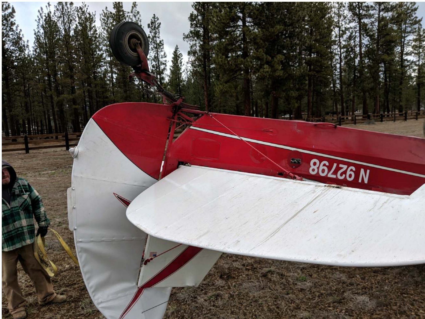
Photo 1 – View of damage to the rudder (Courtesy of FAA)
