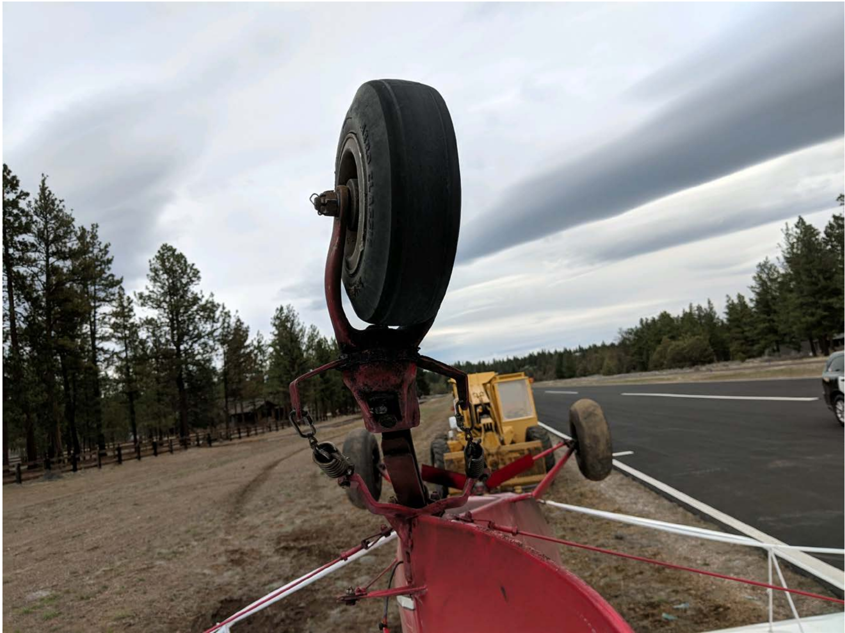
Photo 2 – View of the rudder horns still attached while the airplane is inverted (Courtesy of FAA)
