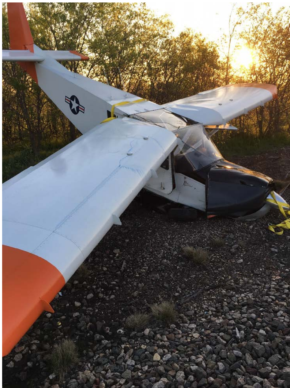
Photo 1 – View of damage to both wings and fuselage (Courtesy of the FAA)
