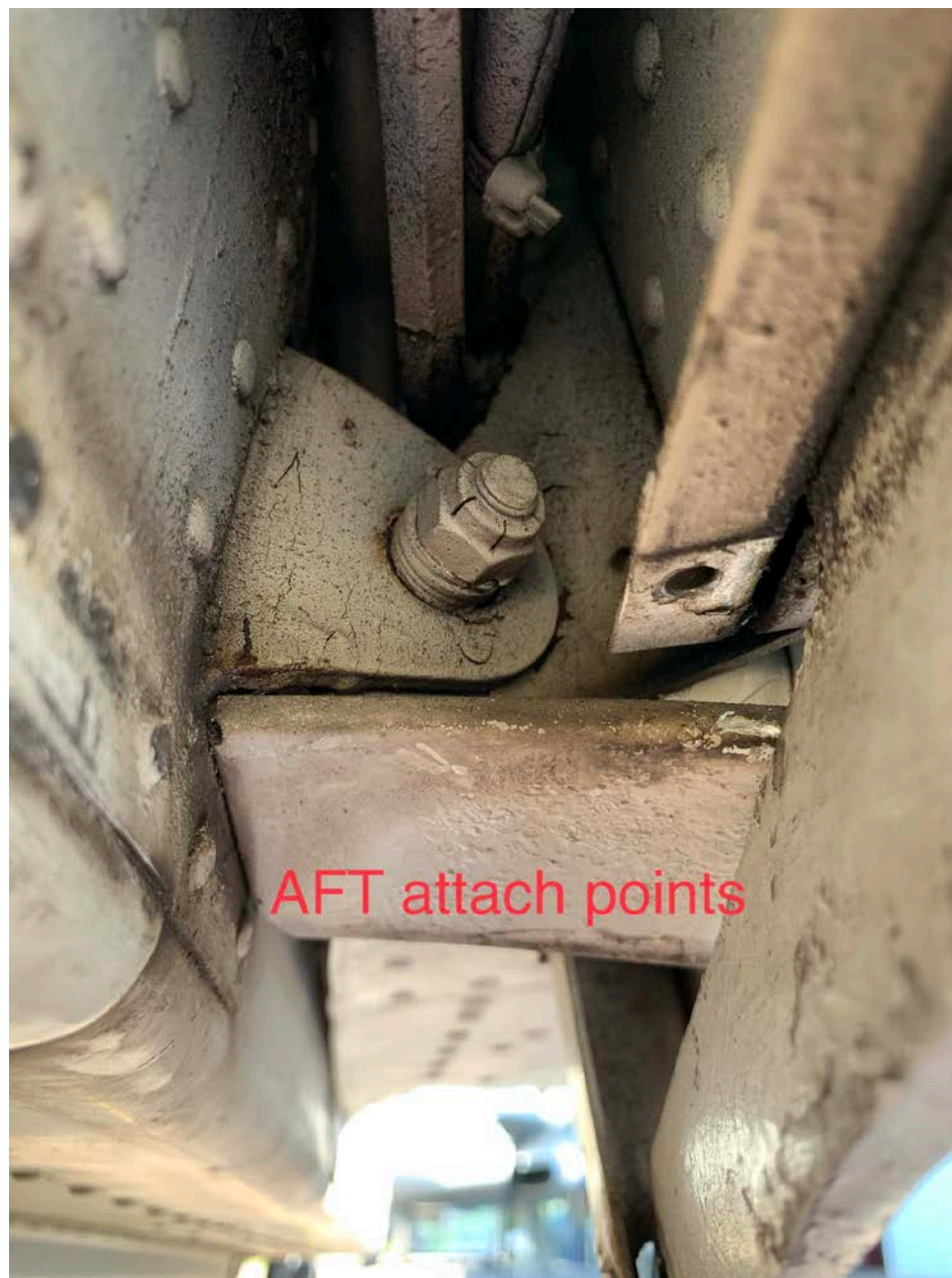
Photo 1 – View facing toward the tail of damage to the aft left wing attachment points (Courtesy of FAA)
