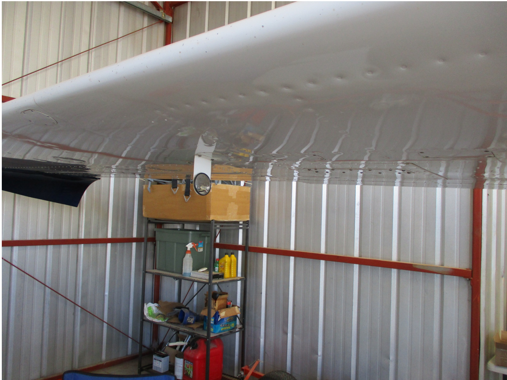
Photo 2 – View of landing gear position observation mirror on right wing (Photo courtesy of the FAA)
