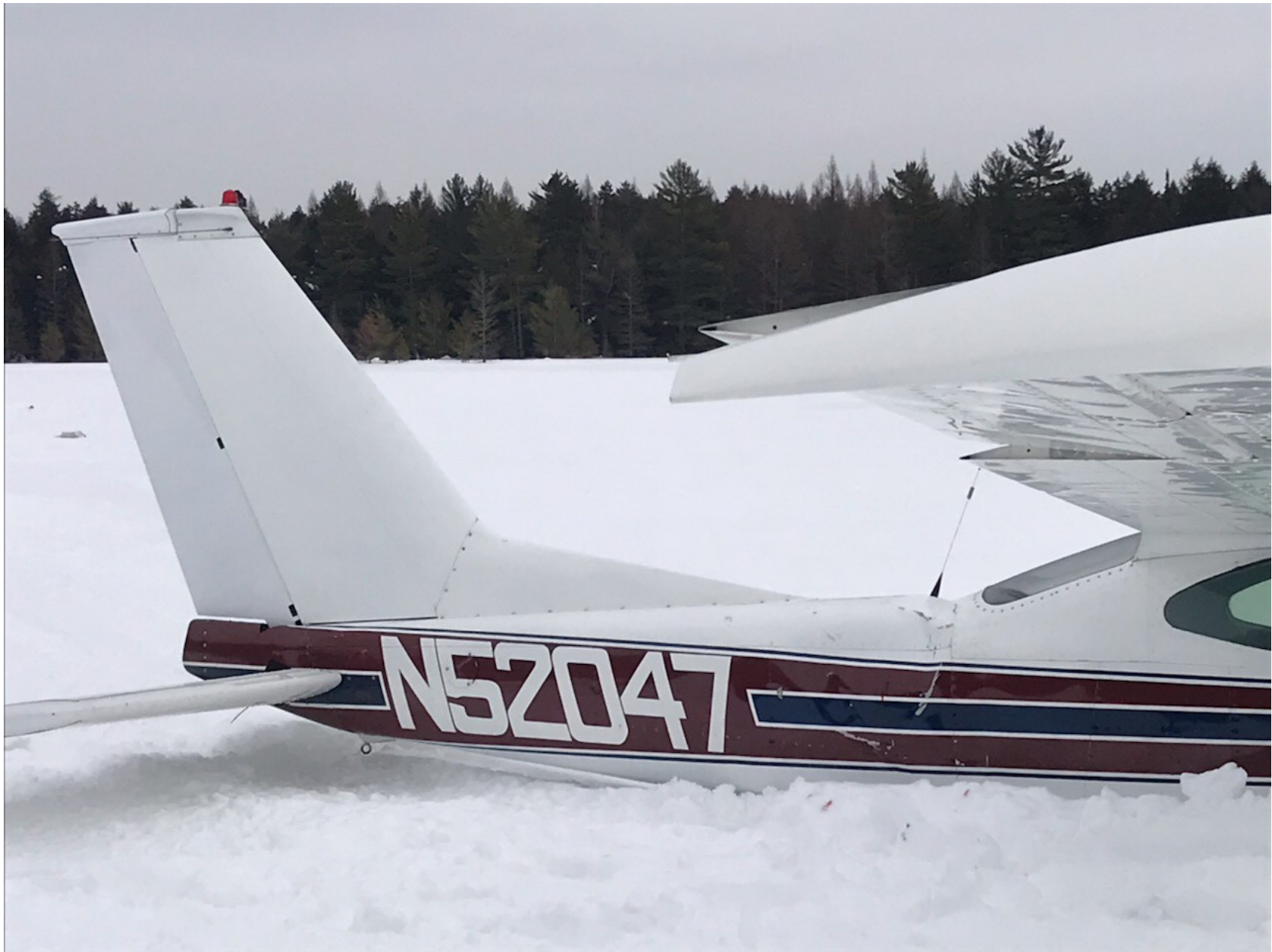
Photo 3 - View of aft fuselage damage (photo courtesy of the FAA)
