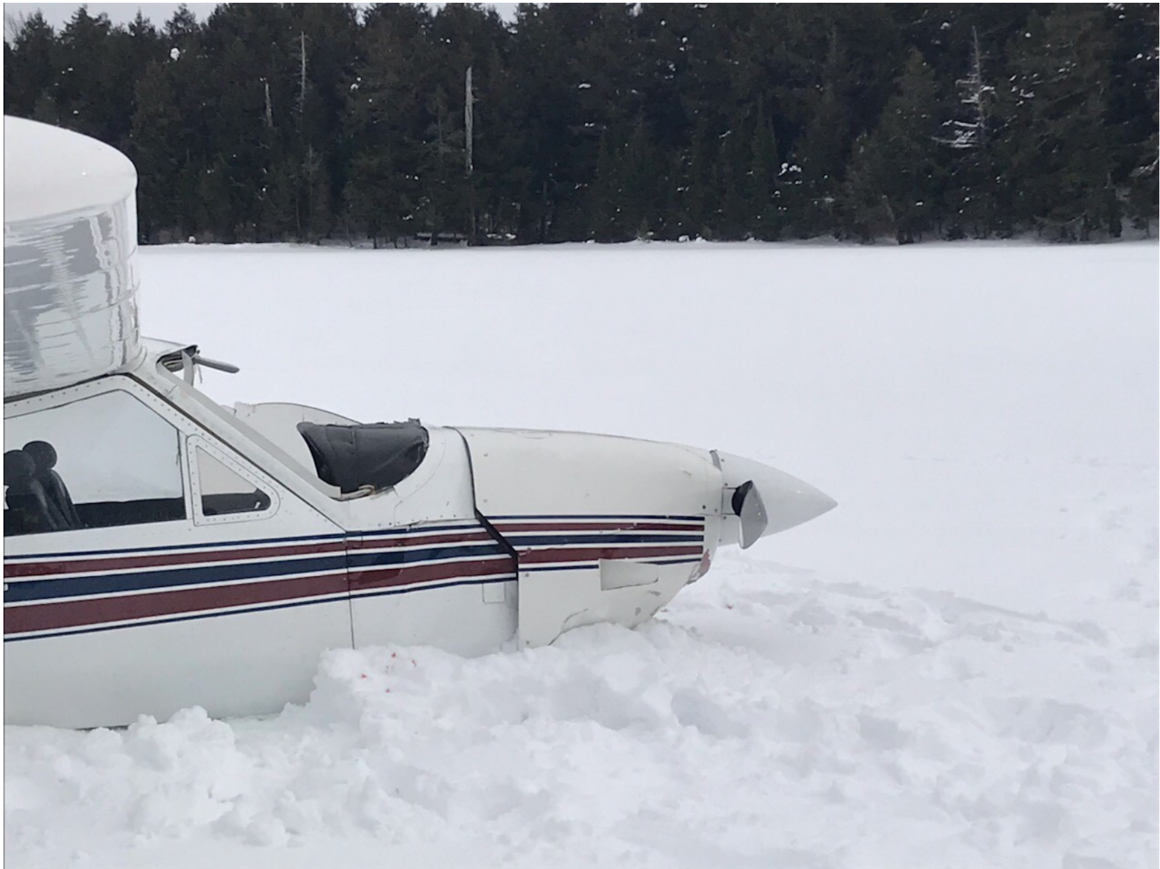
Photo 2 - View of fuselage and cowling damage (photo courtesy of the FAA)
