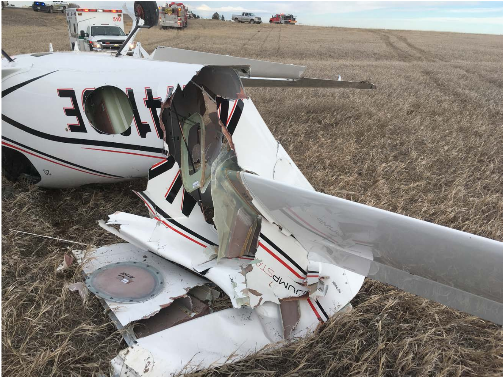
Photo 1 – View of damage to the fuselage and empennage (Courtesy of FAA)
