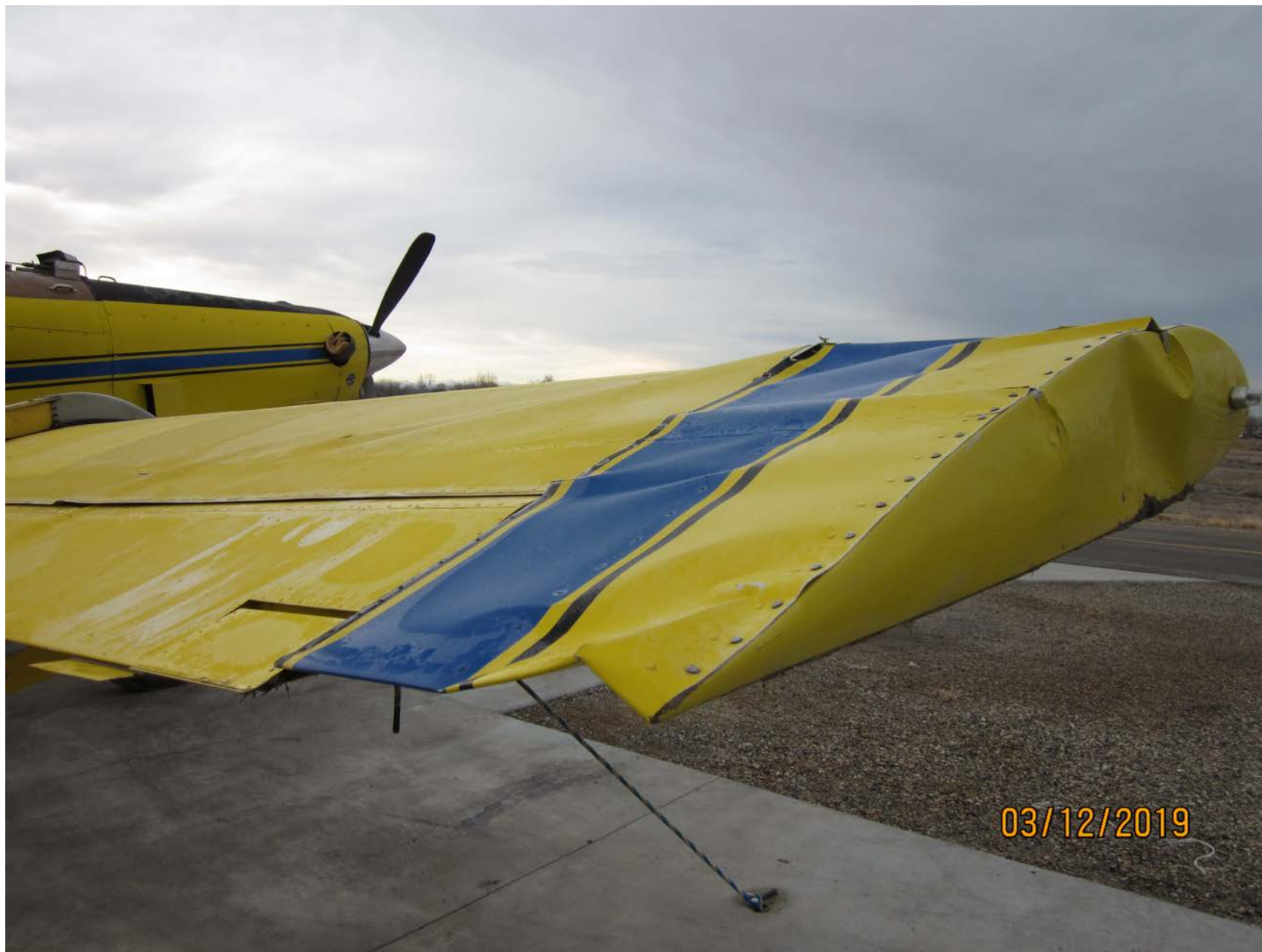
Photo 1 – View of damage to right wing (Courtesy of the FAA)
