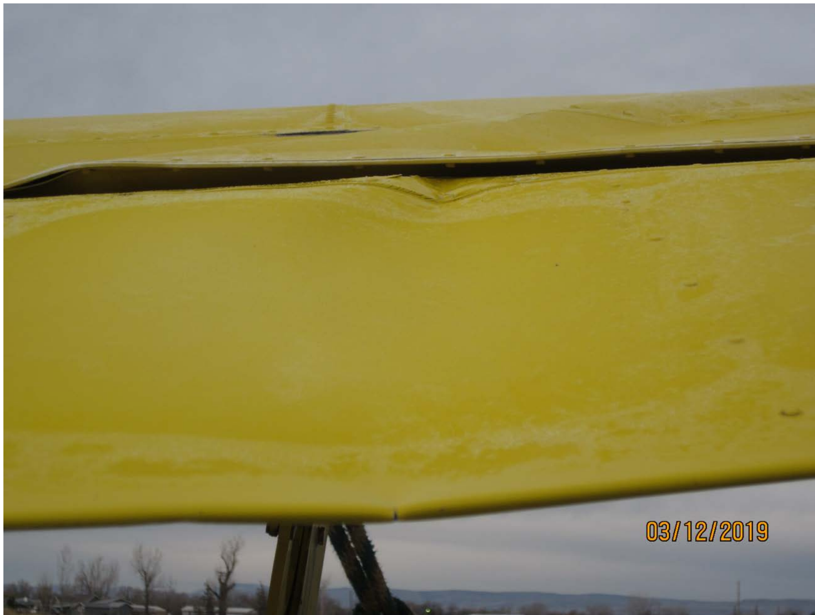
Photo 2 – View of damage to right aileron (Courtesy of the FAA)
