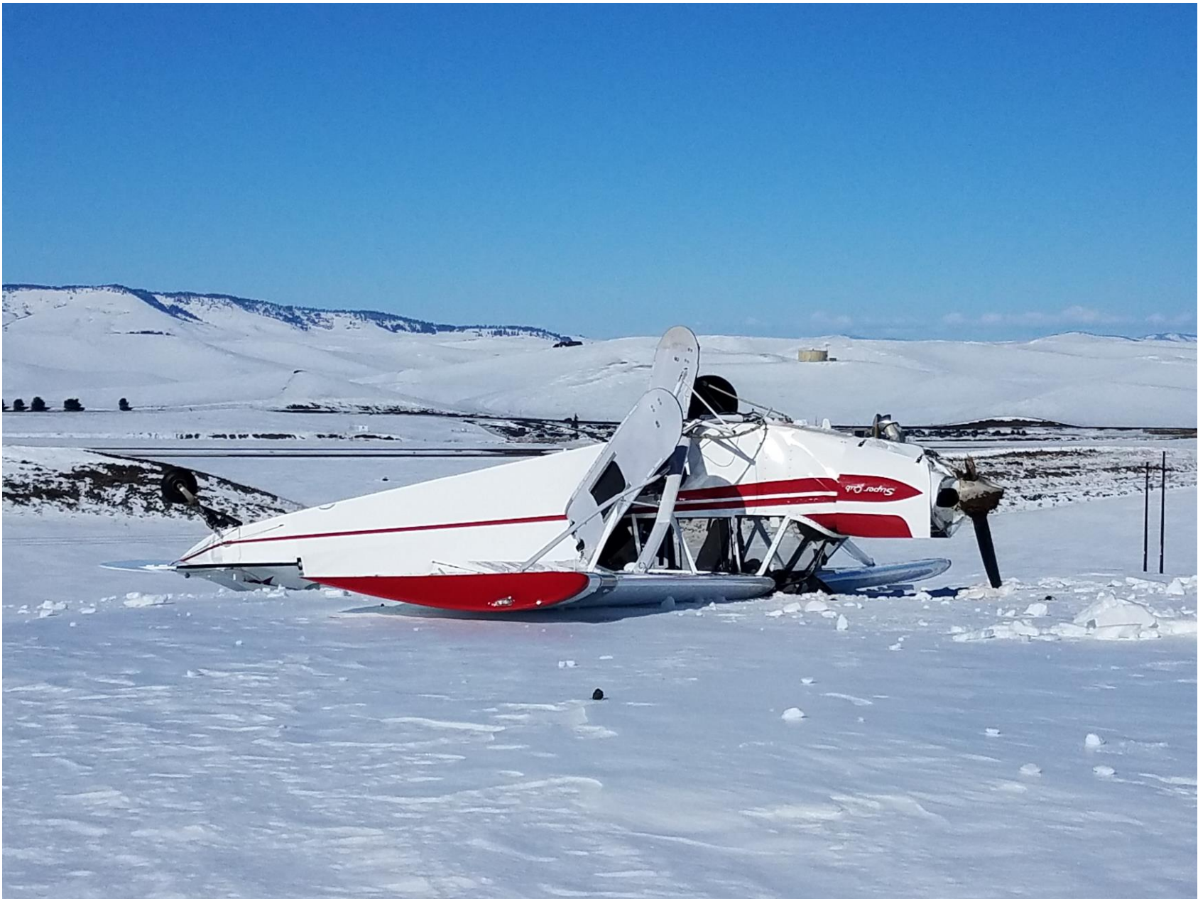
Photo 1 – View of airplane inverted with damaged empennage, fuselage, and lift strut (Photo courtesy of the Sheriff's Office)
