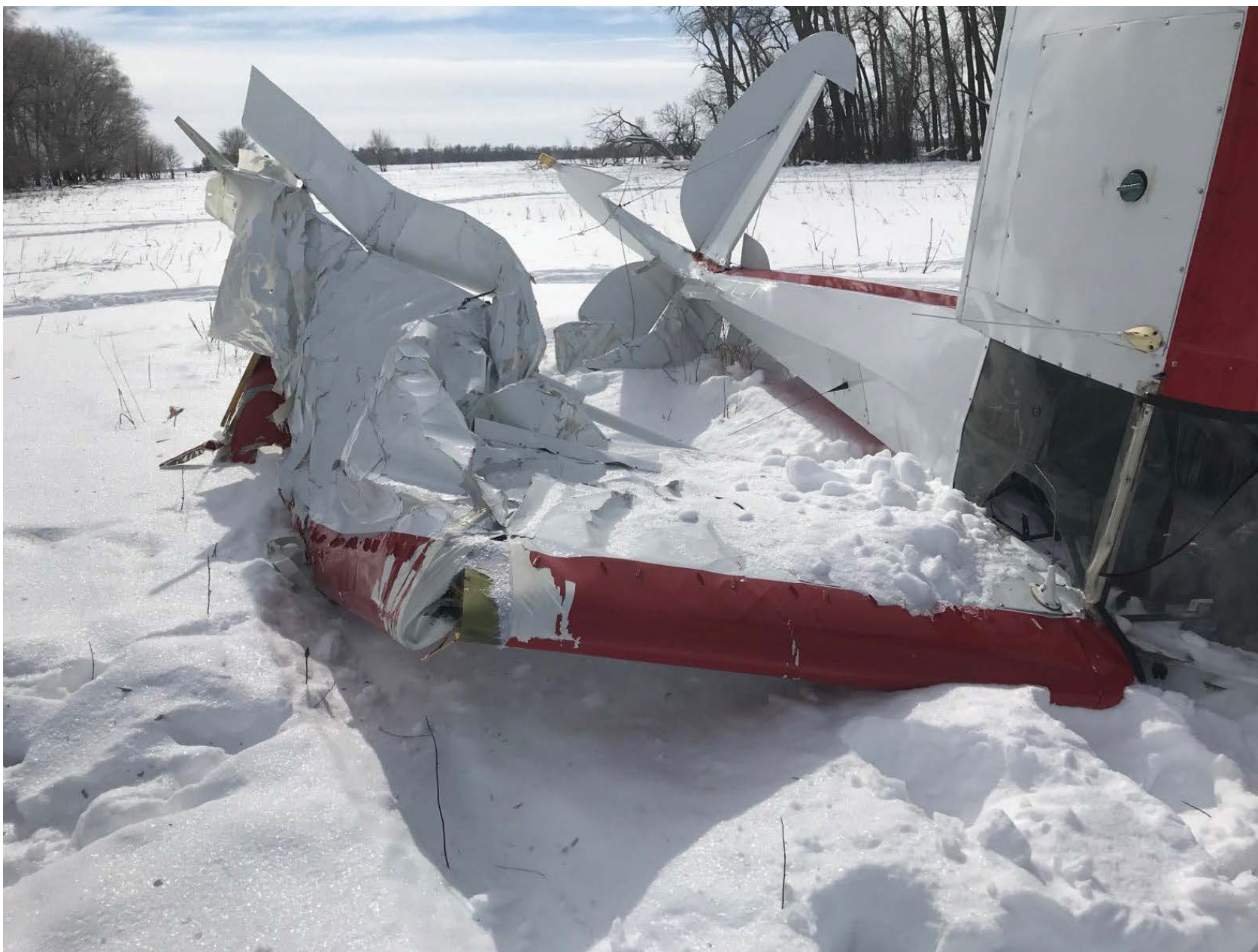
Photo 2 – Close-up view of damaged right wing (courtesy of the FAA)
