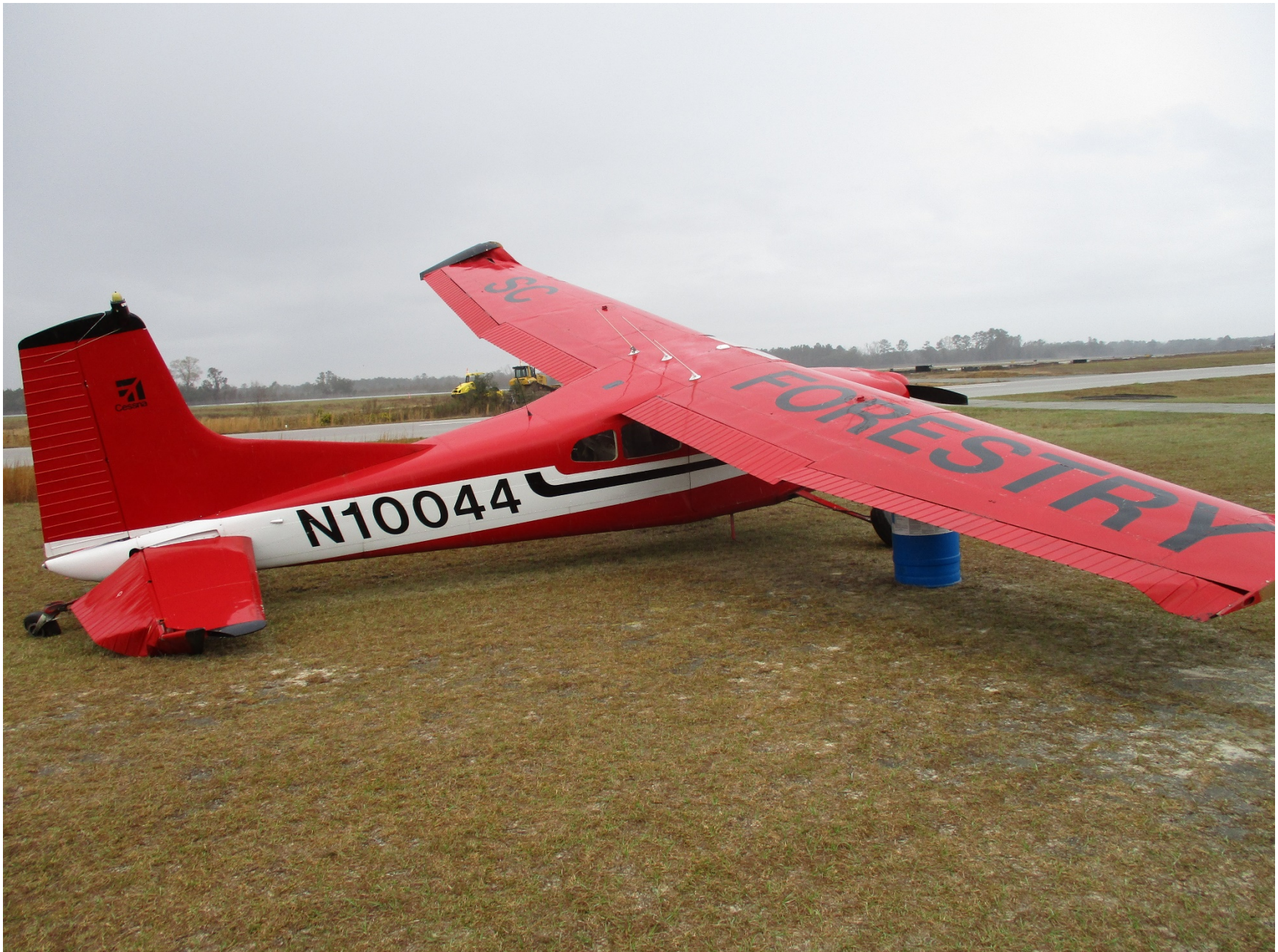
Photo 1 – View of damaged right aileron, right elevator, and left wing (Photo courtesy of the FAA)
