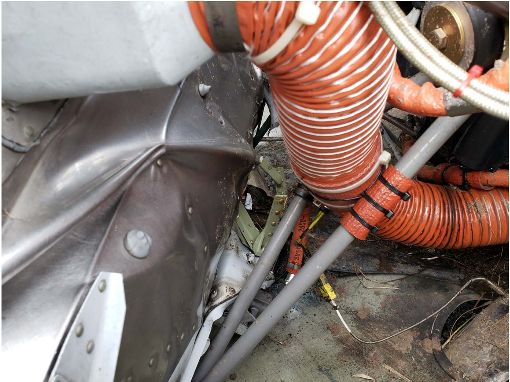
Photo 2 - View of lower engine mount to airframe damage (photo courtesy of the FAA)
