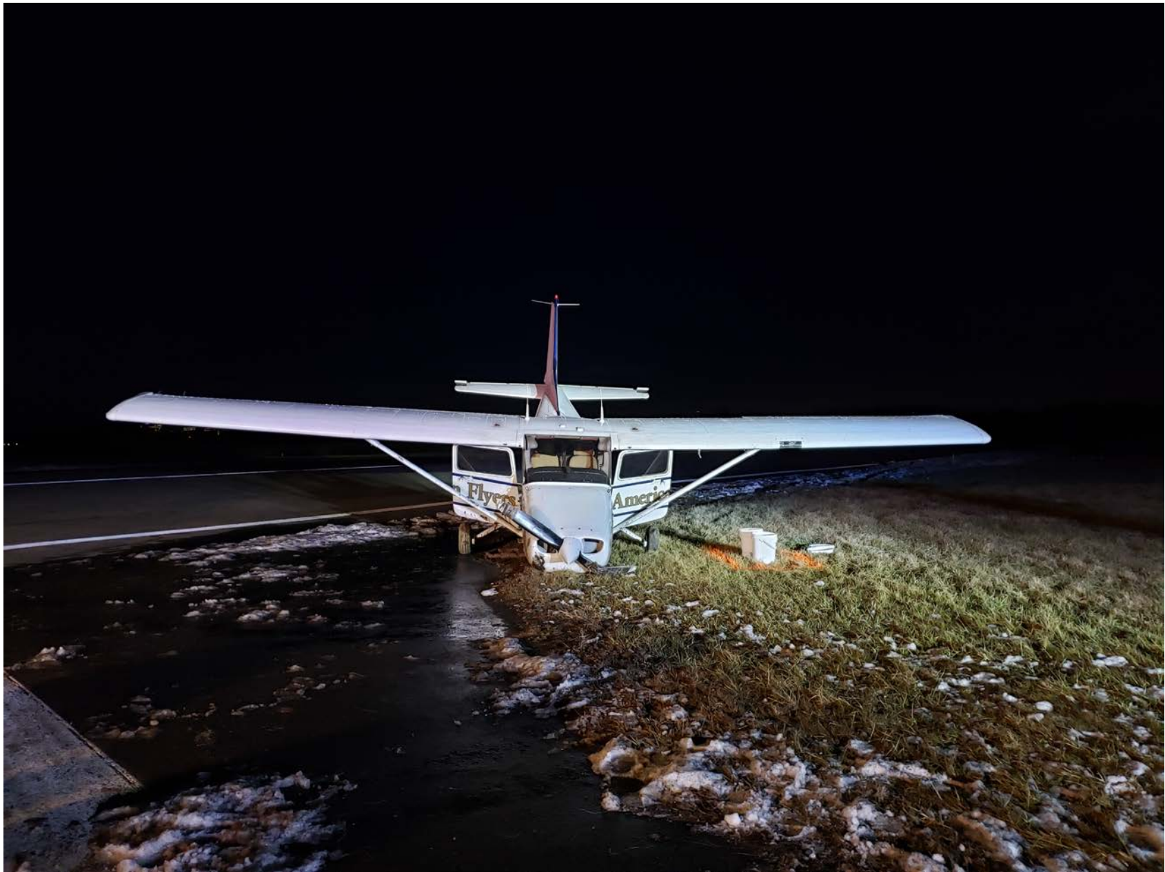
Photo 1 – Front view of fuselage and cowling damage (photo courtesy of the FAA)
