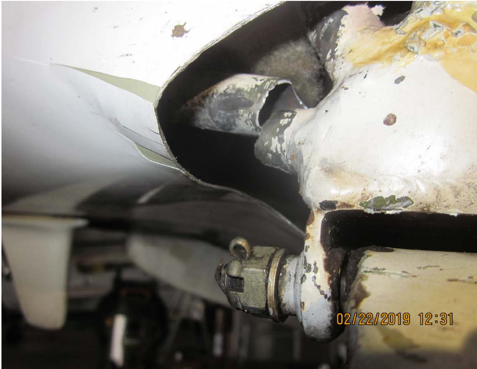
Photo 1 – View of damage to the left main landing gear attachment point (Courtesy of FAA)
