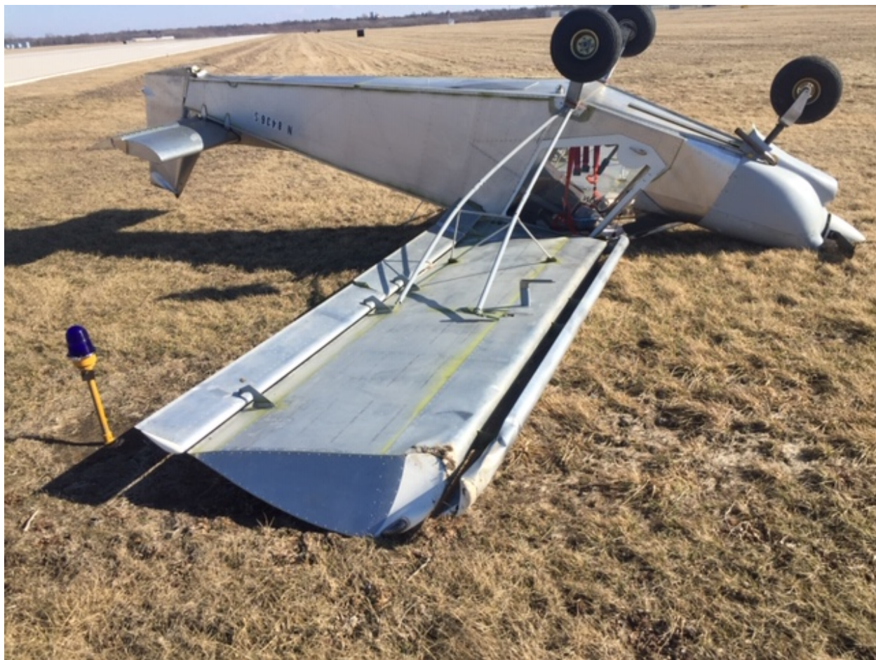
Picture 1 – View of inverted airplane with damaged empennage (Photo courtesy of the FAA)
