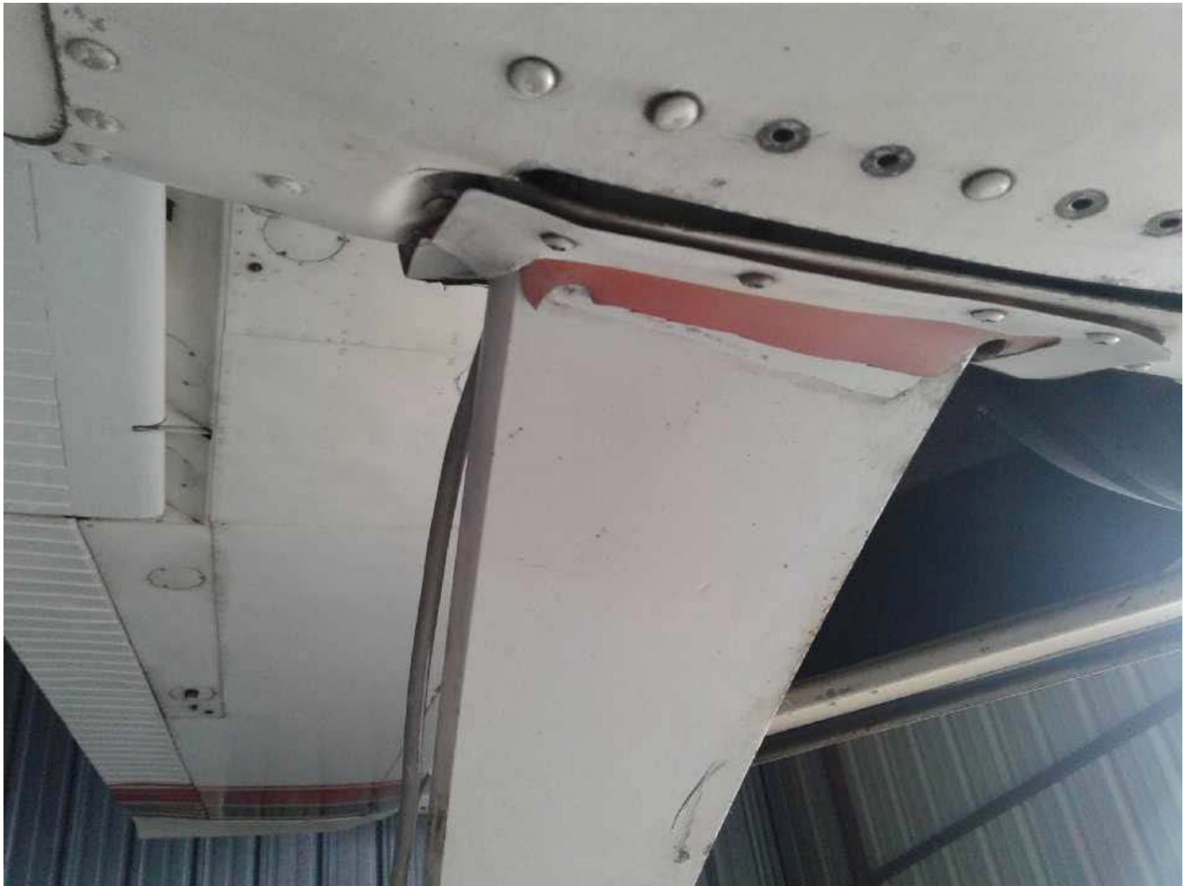
Photo 2 – View of damage to the lower fuselage beneath the left main landing gear attachment points (Courtesy of FAA)
