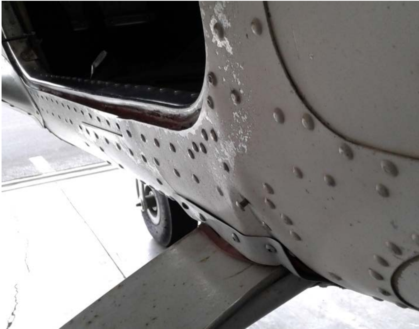
Photo 1 – View of damage to the fuselage above the left main landing gear attachment points (Courtesy of FAA)
