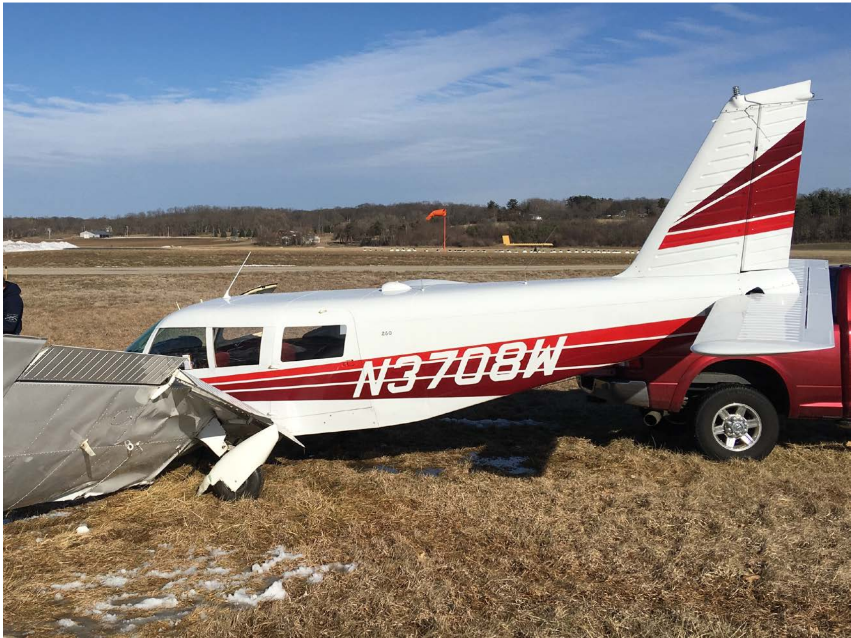
Photo 2 – Aft view of damaged left wing (courtesy of the pilot)
