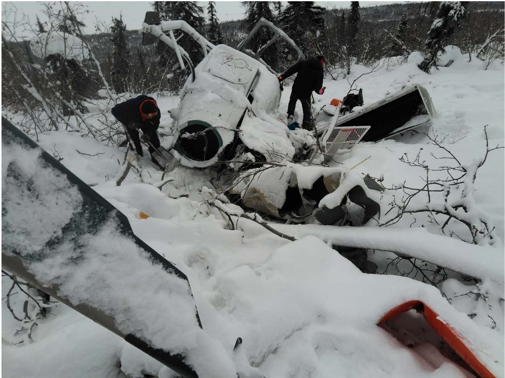
Photo 1 – View of helicopter fuselage, main rotor blades and tail boom damage (courtesy of the operator)
