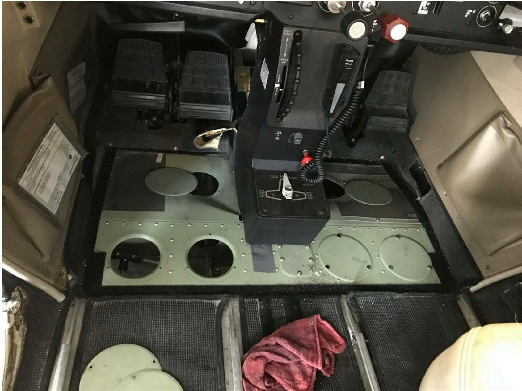
Photo 1 – View of the floorboard portion of the fuselage damage (photo courtesy of flight school)
