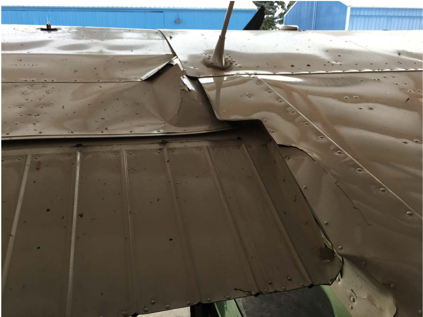
Photo 2 – View of damage to the left wing root of N9101X (Courtesy of FAA)
