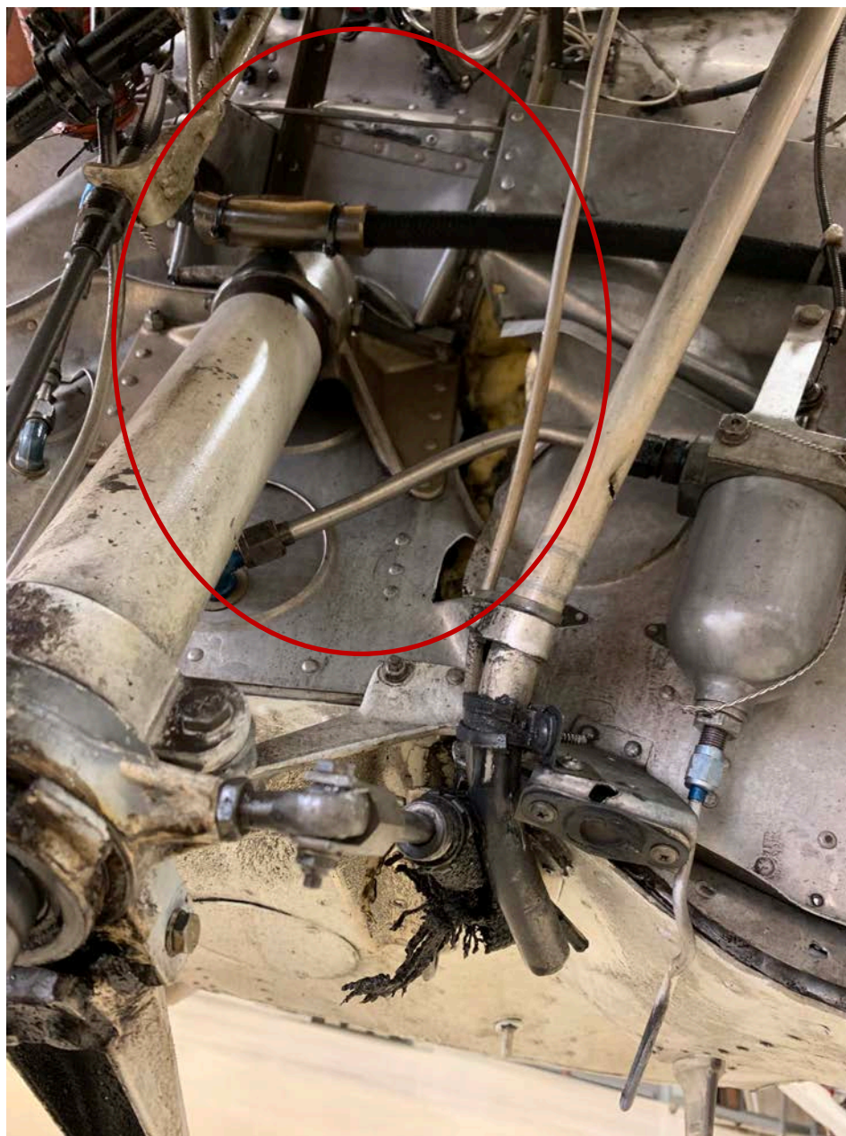
Photo 2 – View of damage to firewall and nose landing gear tunnel (courtesy of the airframe and powerplant mechanic)
