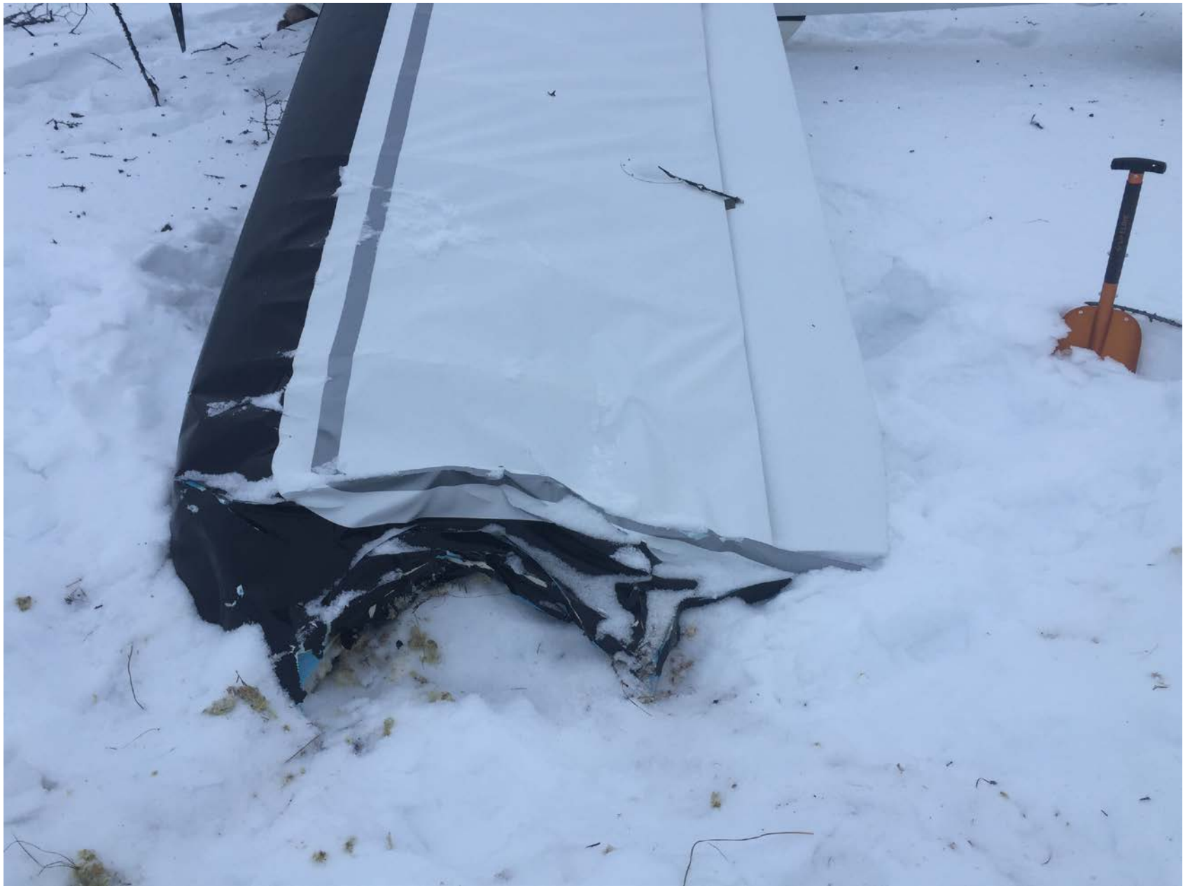
Photo 1 – View of left wing damage (photo courtesy of FAA)
