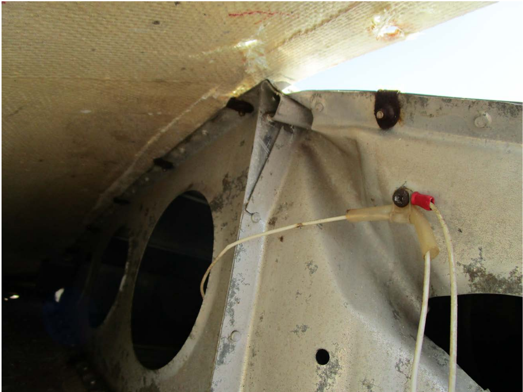
Photo 2 – View of damage to the outboard right rib wing nose (Courtesy of FAA)
