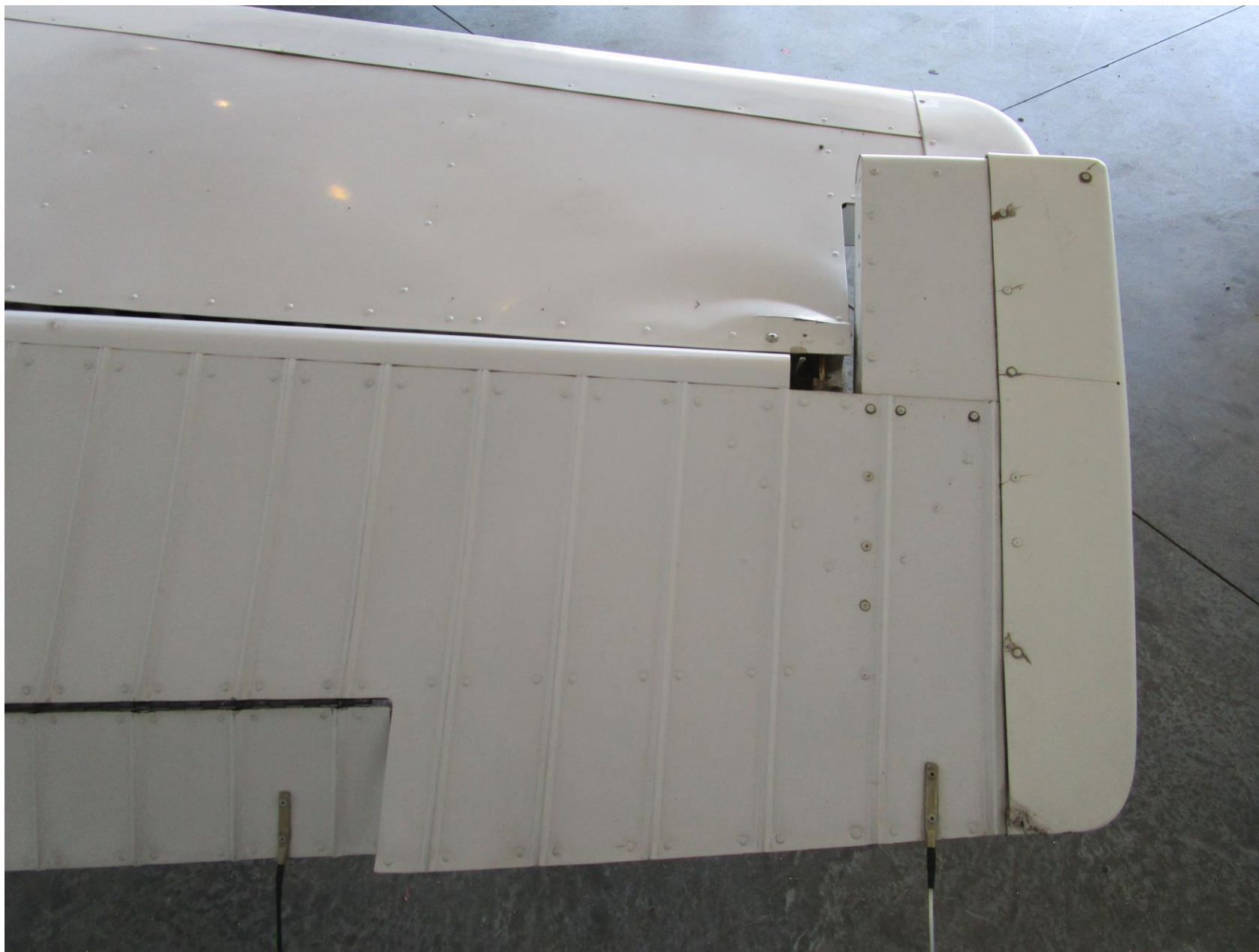
Photo 2 – View of damaged right horizontal stabilizer (Photo courtesy of the FAA)
