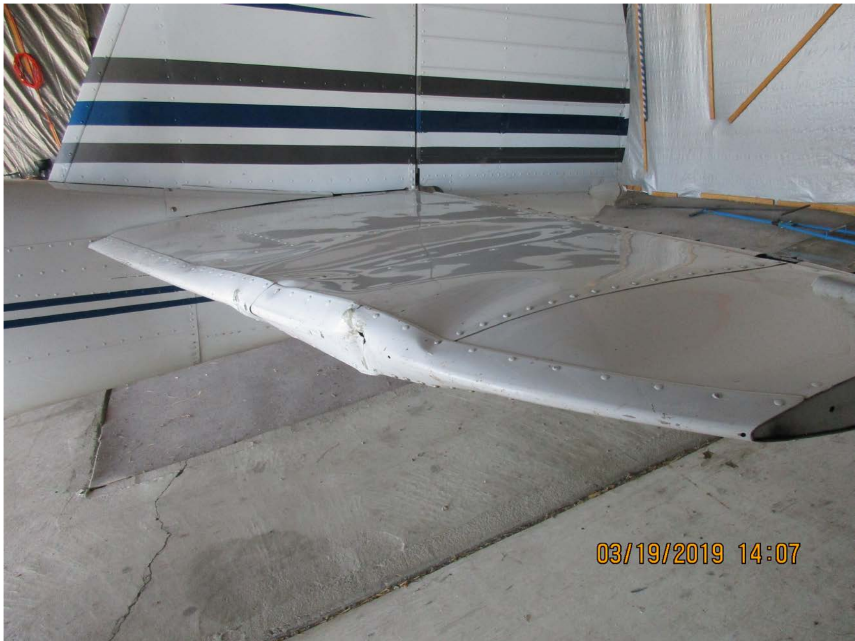
Photo 1 – View of damage to the left horizontal stabilizer (Courtesy of FAA)
