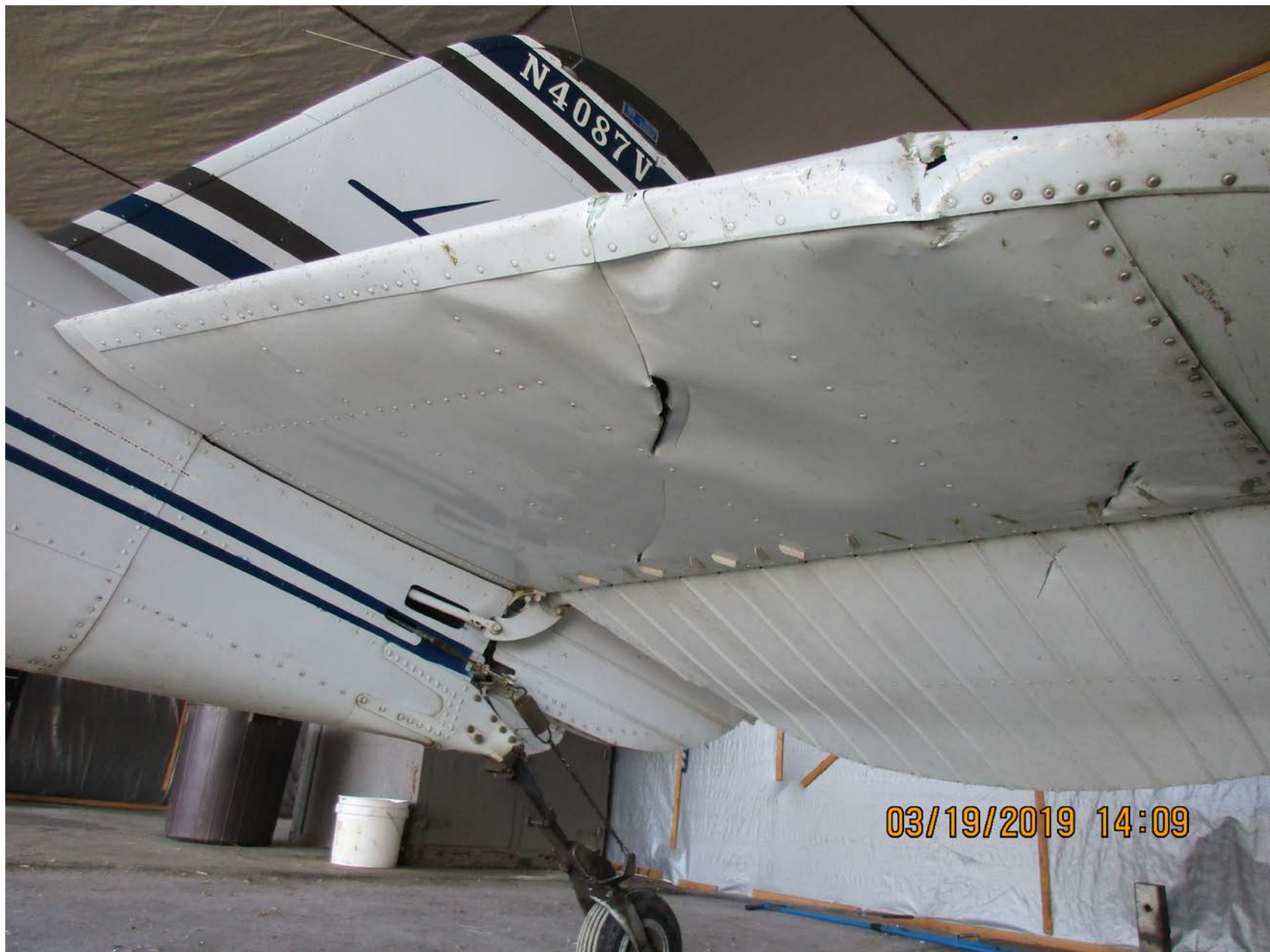
Photo 2 – View of damage to the bottom of the left horizontal stabilizer (Courtesy of FAA)
