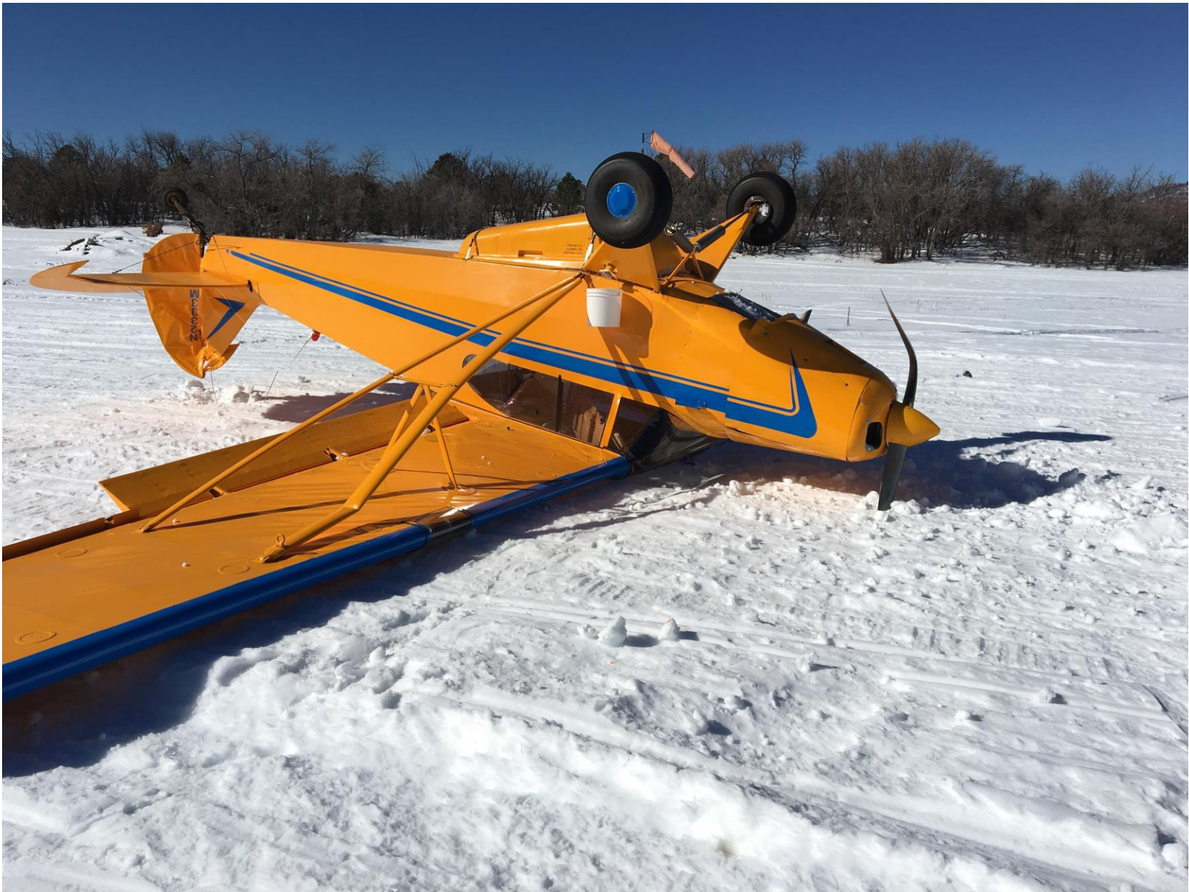
Photo 1 – View of inverted airplane with damaged left wing lift strut and empennage (Photo courtesy of unknown)
