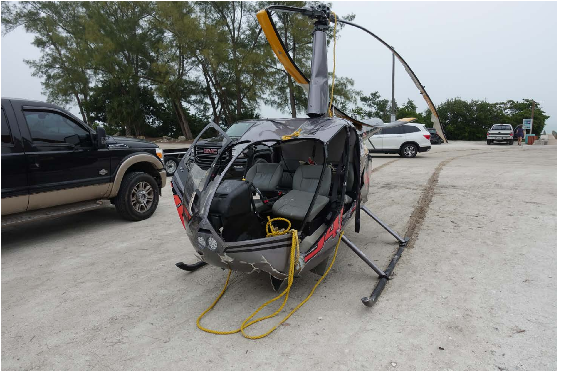
Photo 1 – View of damaged main rotor blades and fuselage (courtesy of the FAA)
