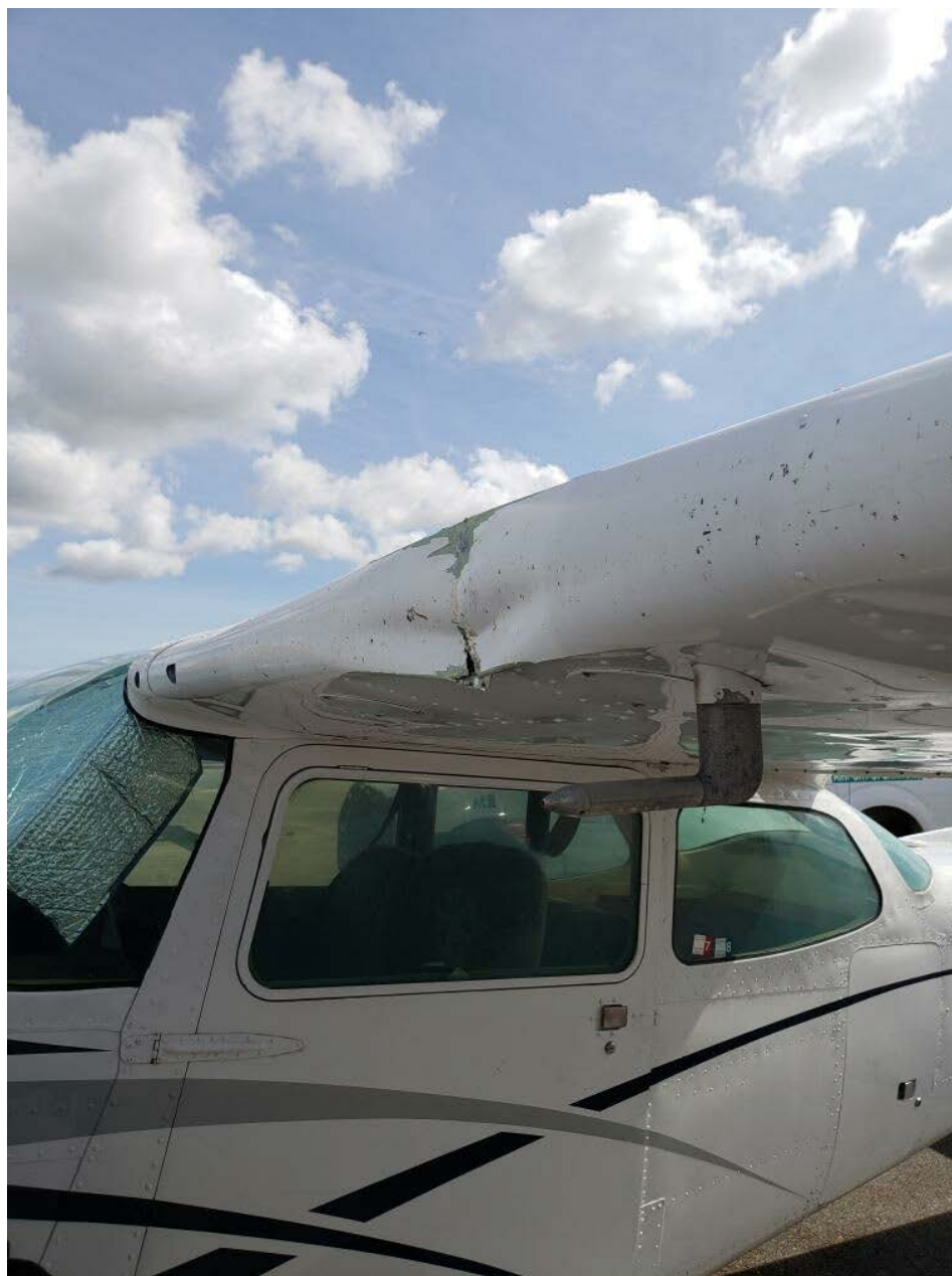
Photo 1 – View of damage to the left wing (Courtesy of FAA)
