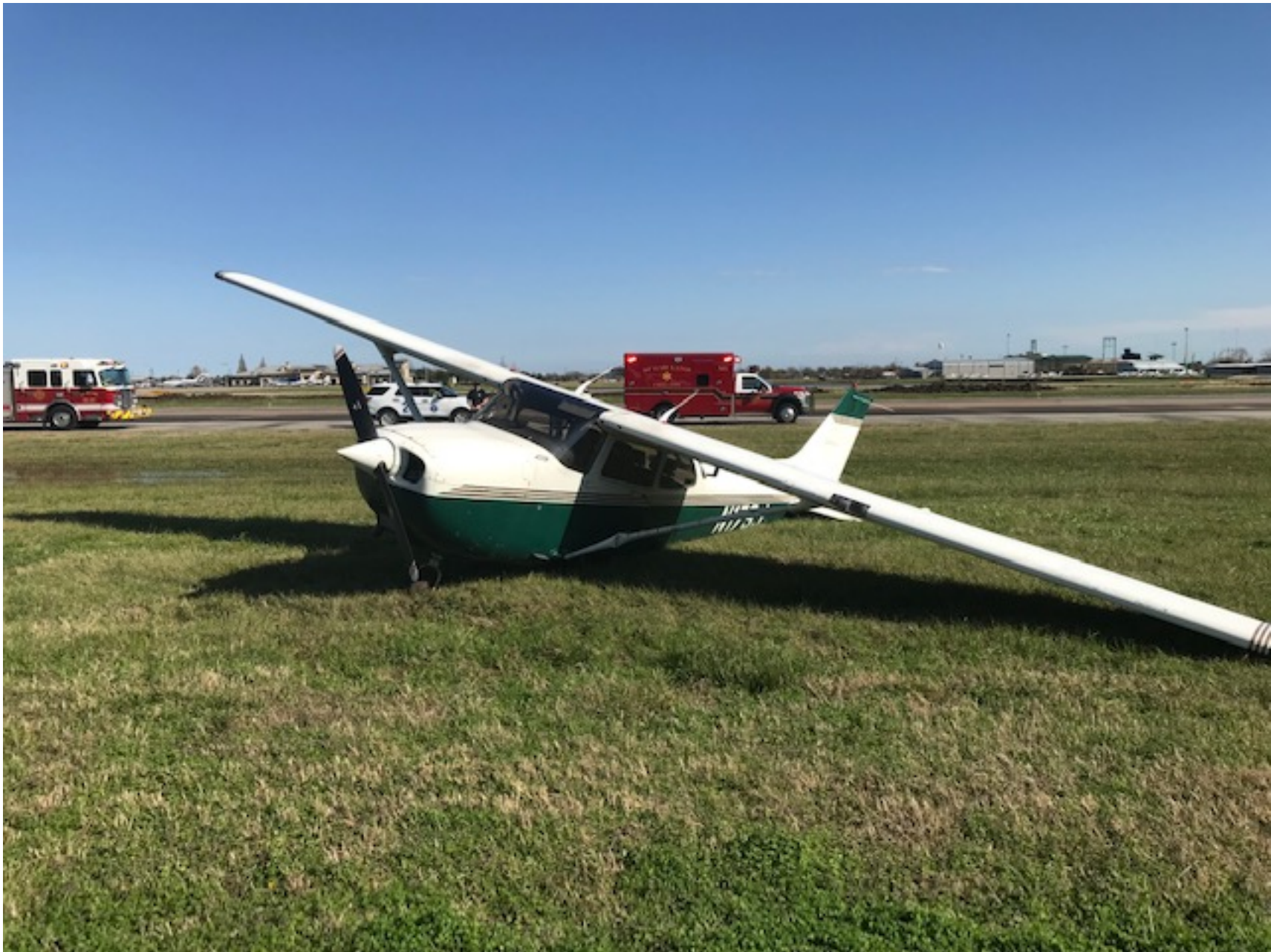
Photo 2 – View of damaged left wing lift strut (Photo courtesy of the FAA)
