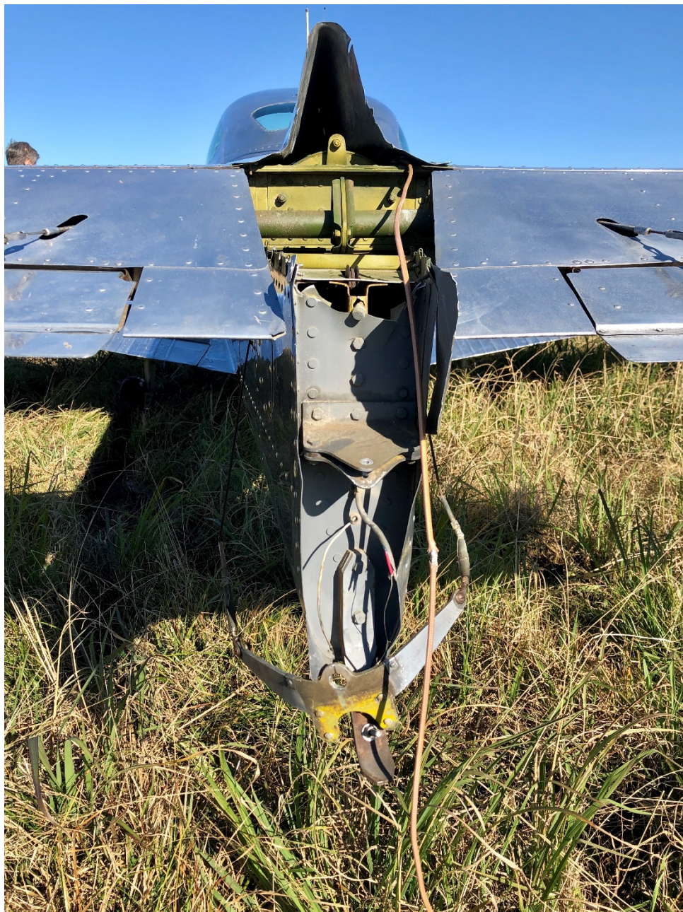
Photo 2 – View of damaged empennage from rear (Photo courtesy of the pilot)
