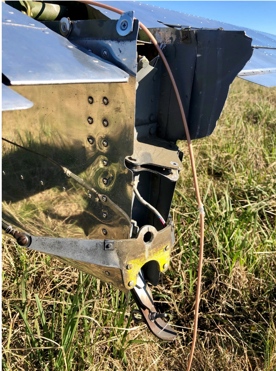
Photo 3 – View of damaged empennage (Photo courtesy of the pilot)
