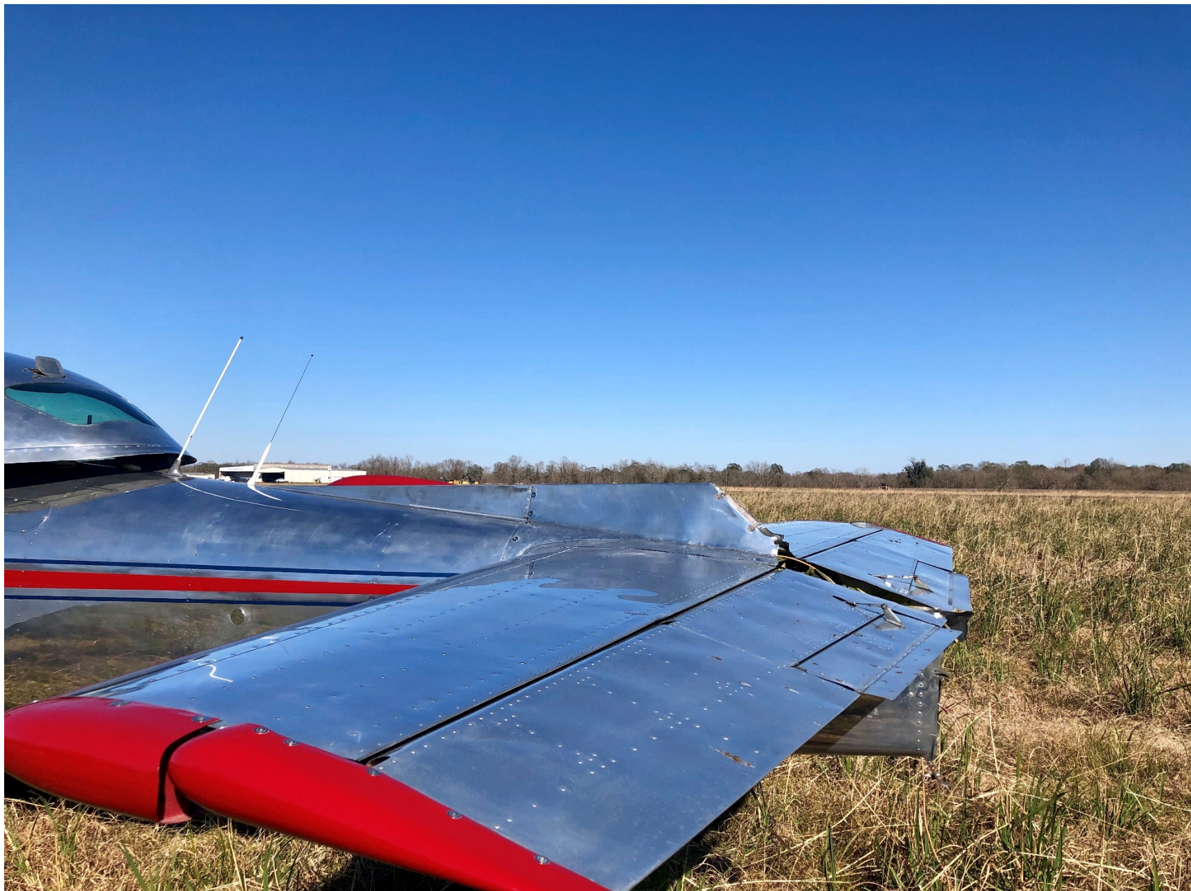
Photo 1 – View of damaged empennage without vertical stabilizer and rudder (Photo courtesy of the pilot)
