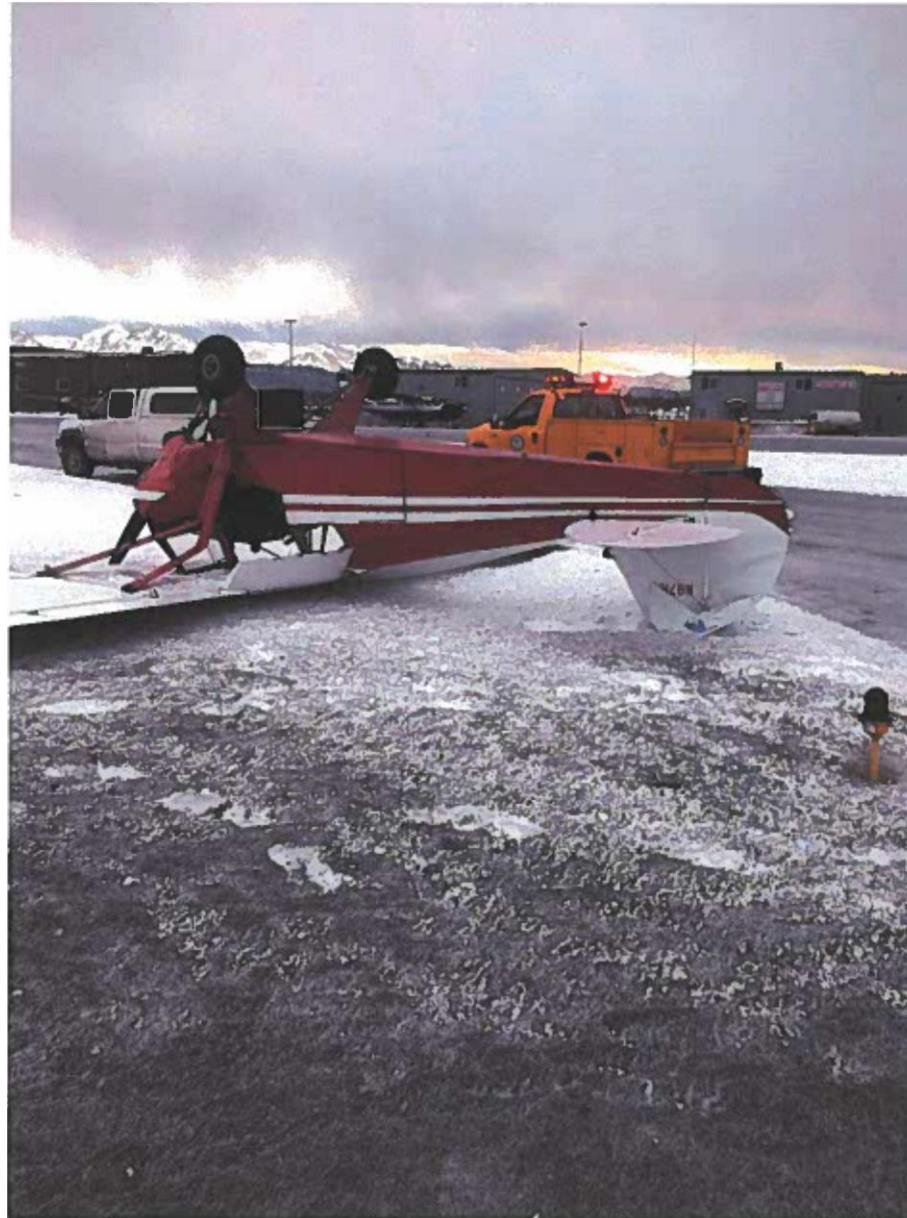
Photo 1 - View of airplane inverted with damage to the right wing lift strut and empennage (Photo courtesy of unknown)
