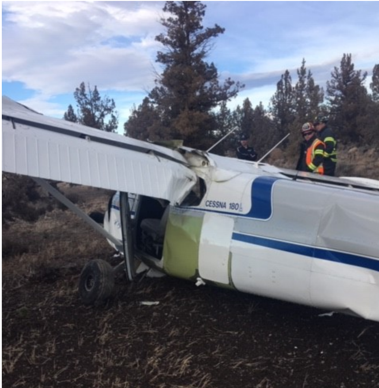
Photo 3 - View of left wing damage (photo courtesy of law enforcement)
