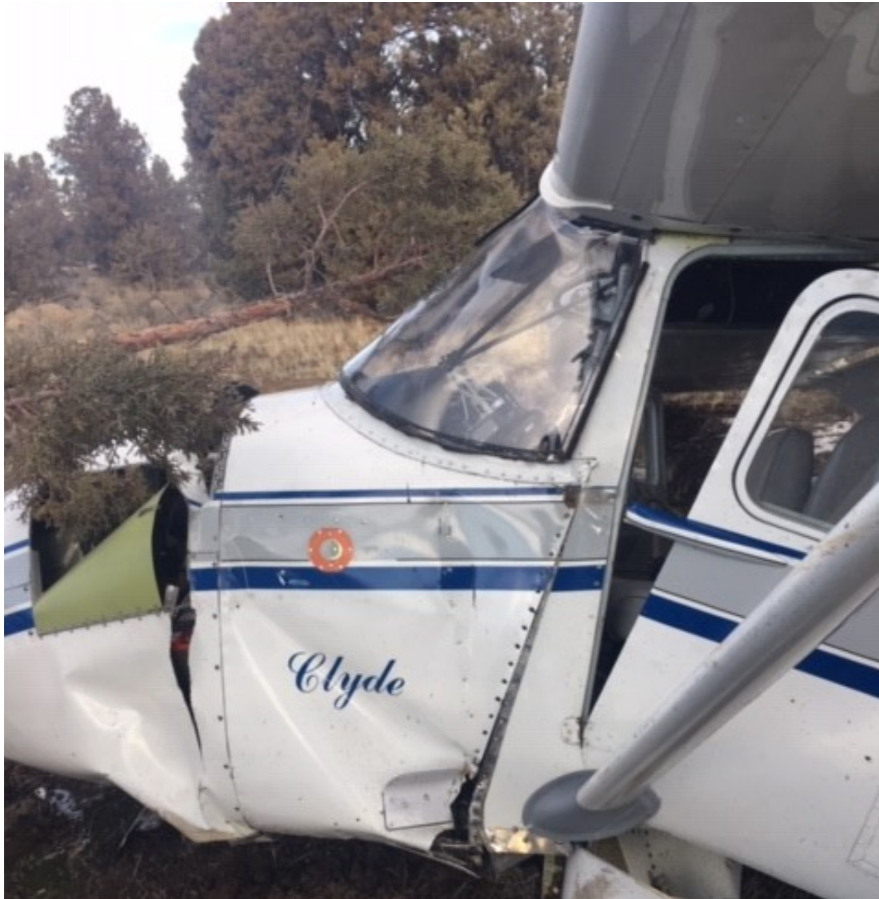
Photo 4 – View of fuselage damage (photo courtesy of law enforcement)
