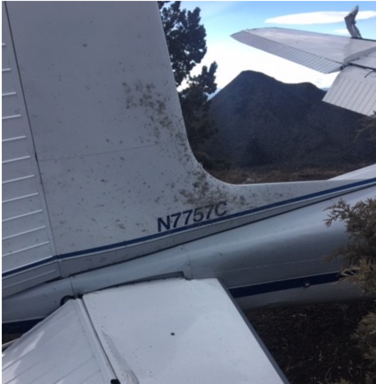
Photo 1 – View of elevator damage (photo curtesy of law enforcement)
