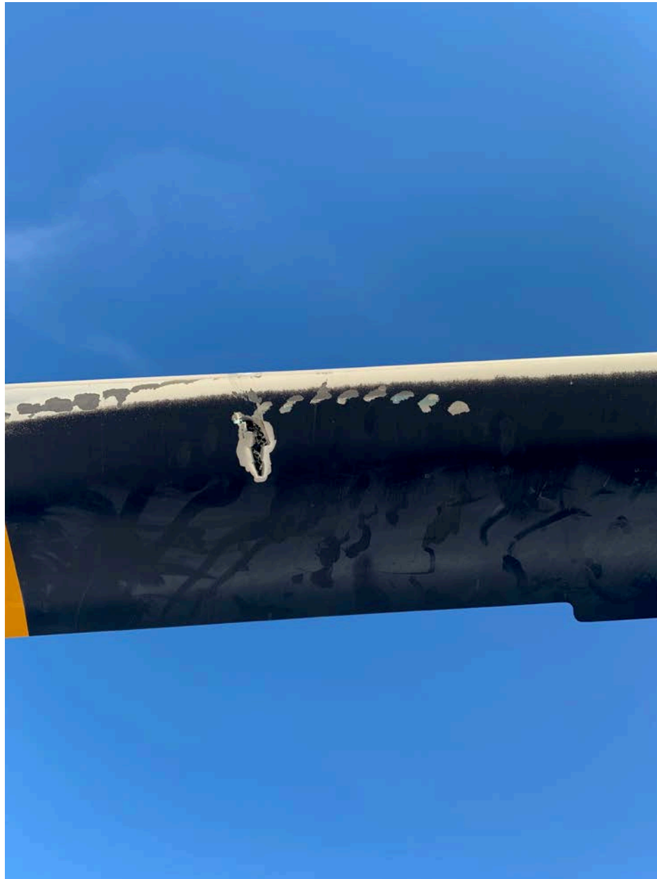
Photo 3 - View of main rotor damage (photo courtesy of the FAA)
