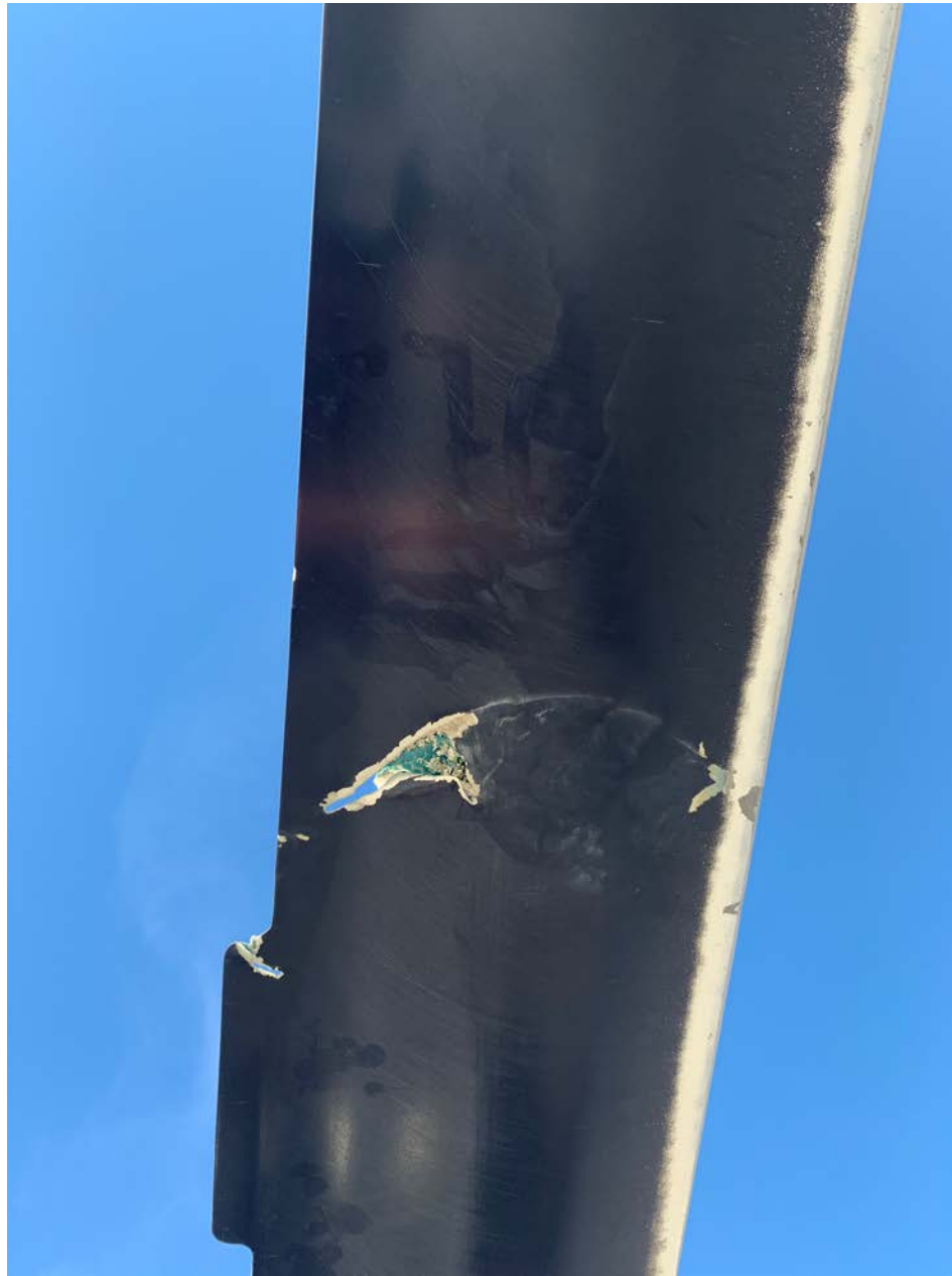
Photo 1 – View of main rotor damage (photo courtesy of the FAA)
