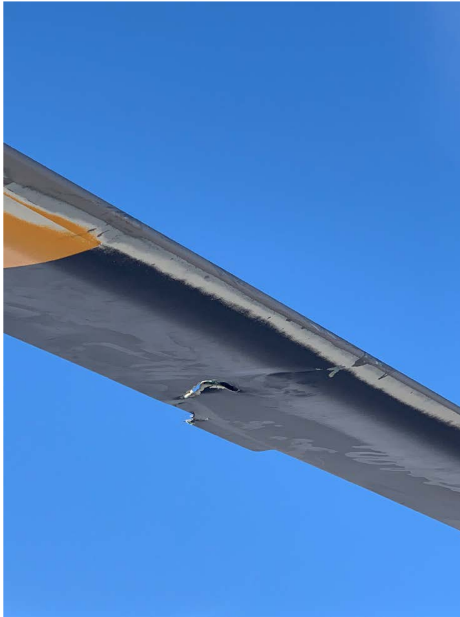
Photo 2 - View of main rotor damage (photo courtesy of the FAA)
