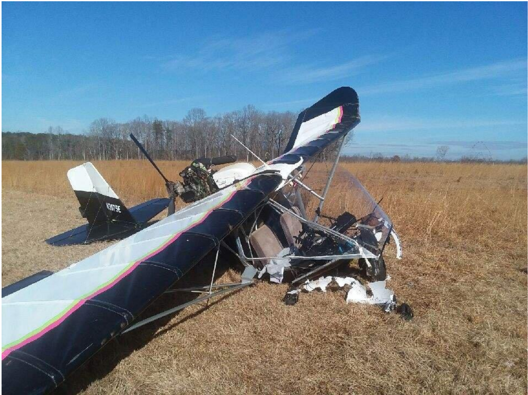
Photo 1 – View of right, front fuselage damage (photo courtesy of the FAA).
