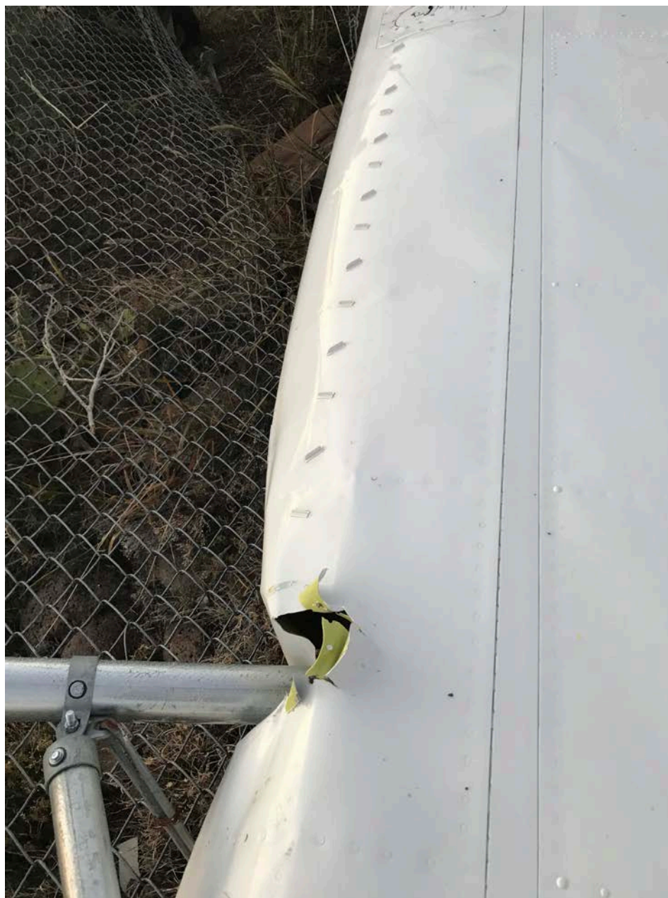
Photo 1 – View of damage to the leading edge of the left wing (Courtesy of FAA)
