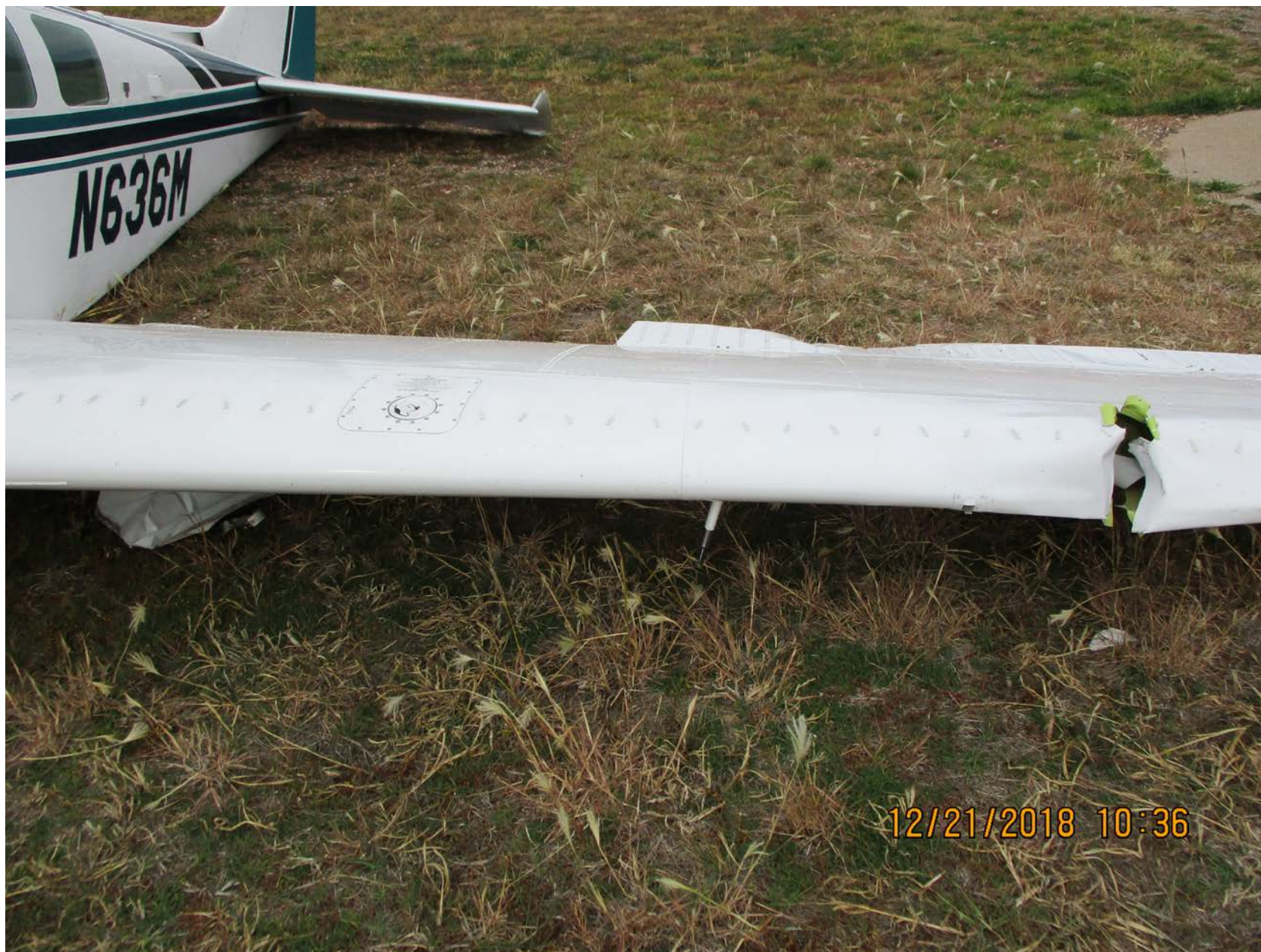
Photo 2 – View of damage to the left wing and aileron (Courtesy of FAA)
