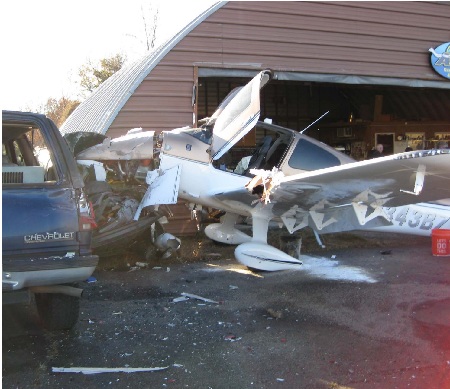
Photo 1 – View of damaged fuselage and left wing after impacting building (Photo courtesy of the FAA)
