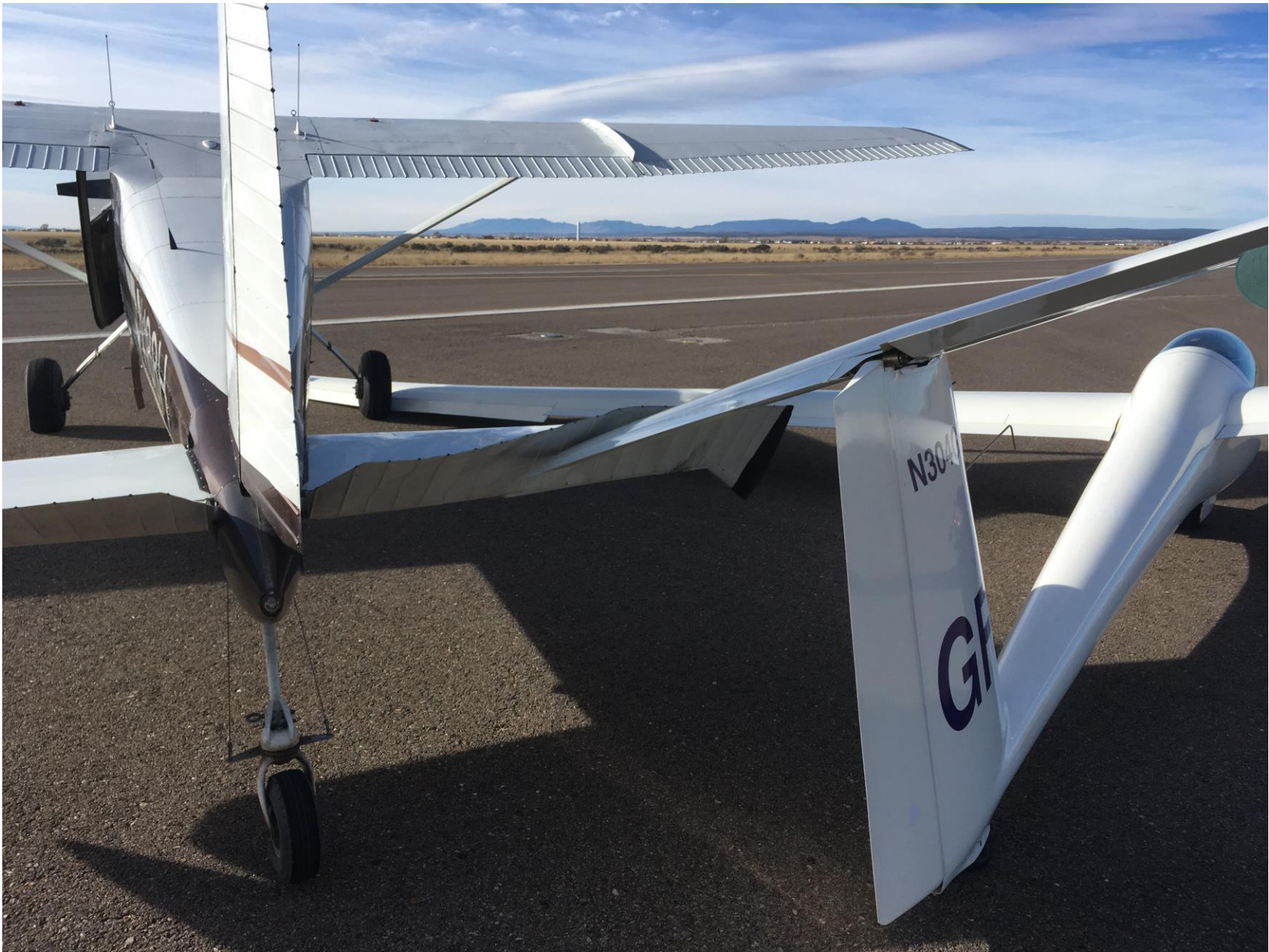
Photo 1 – View of right elevator damage (photo courtesy of the FAA)
