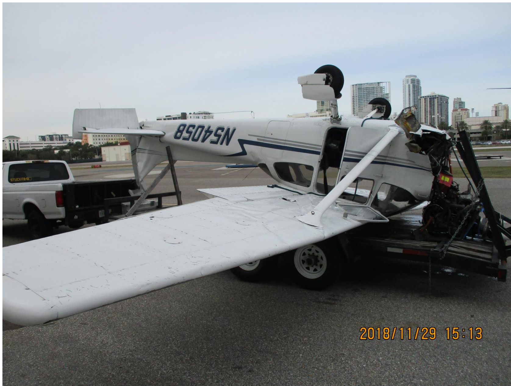
Photo 1 – View of damaged fuselage and empennage (Photo courtesy of the FAA)
