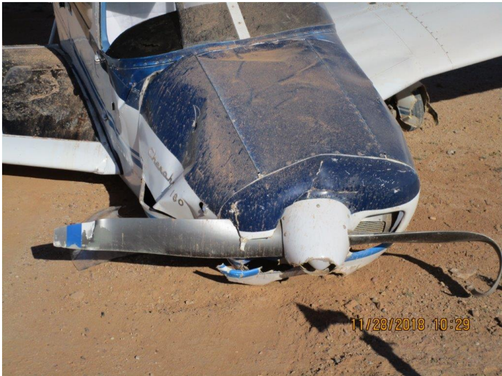
Photo 2 – View of damaged forward fuselage (courtesy of the FAA)
