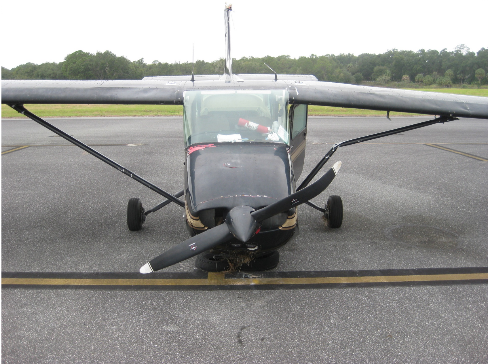
Photo 1 – View of damaged left wing lift strut (Photo courtesy unknown)
