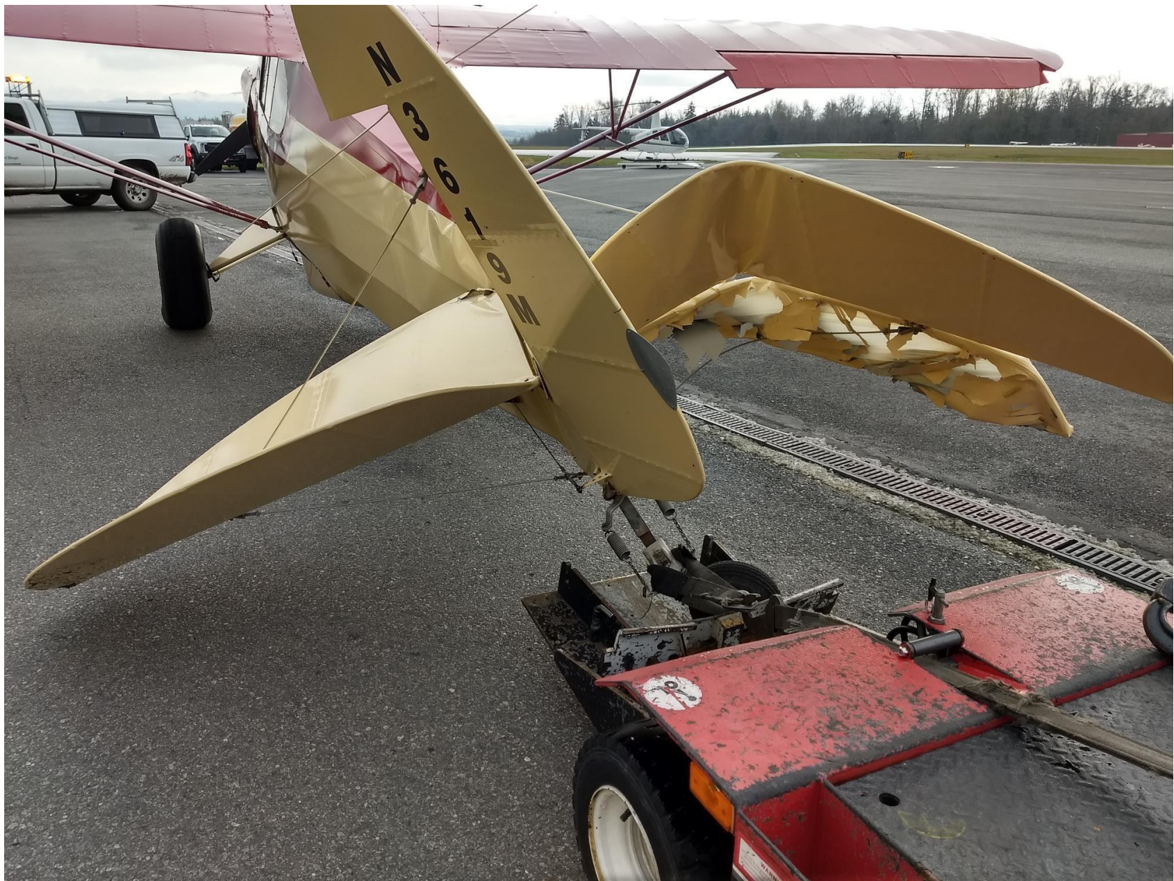
Photo 1 – Rear view of damaged empennage and fuselage (Photo courtesy of unknown)
