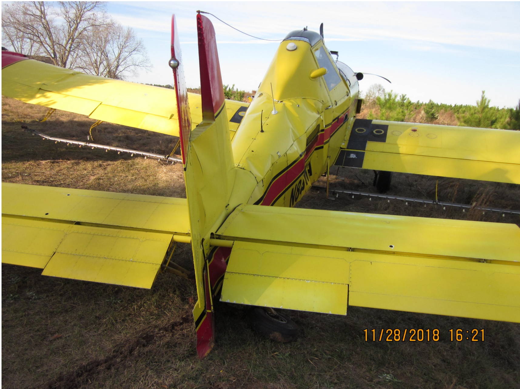
Photo 1 – View of fuselage damage from rear of airplane (Photo courtesy of the FAA)
