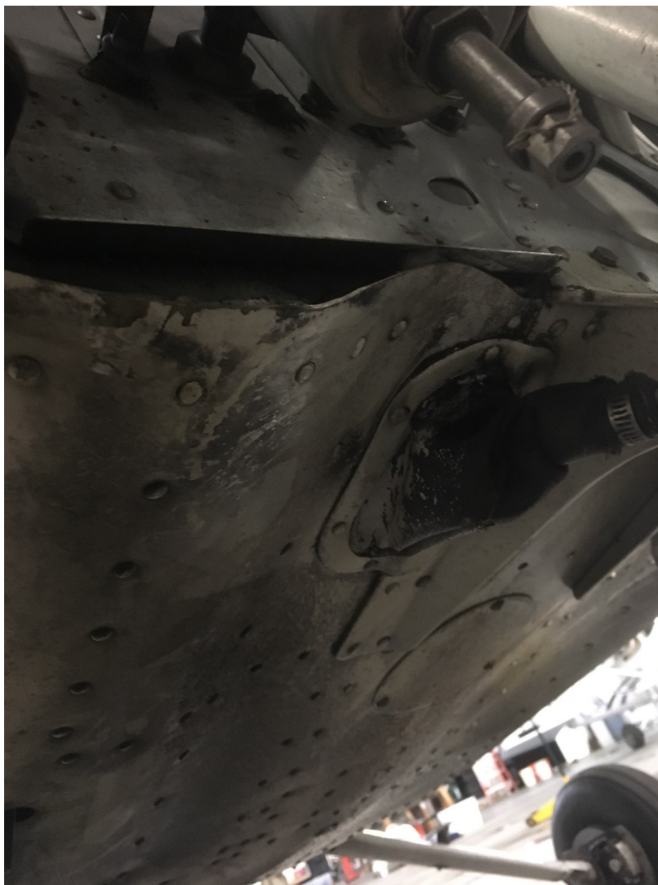
Photo 2 – View of damaged lower fuselage (Photo courtesy of the FAA)
