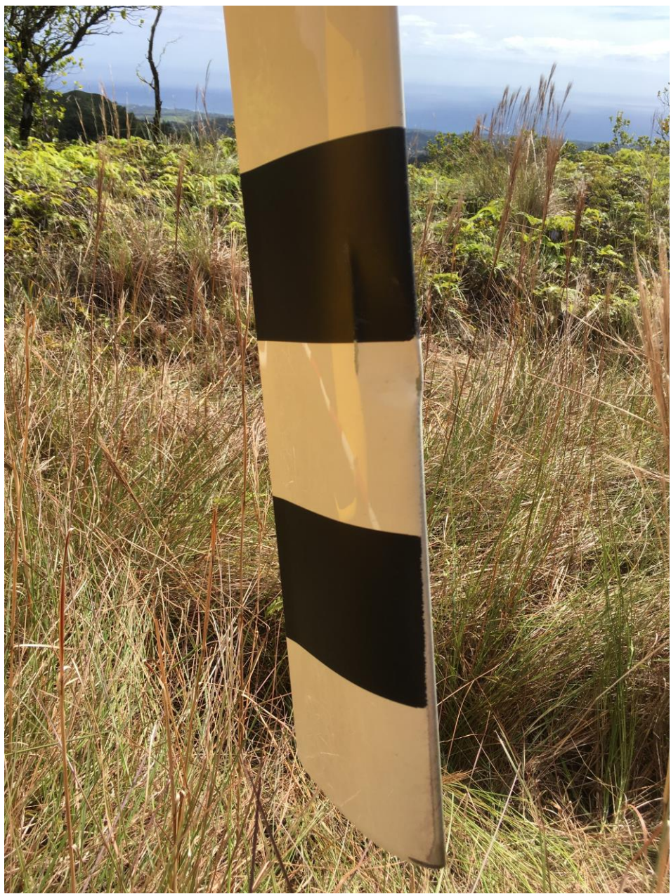
Photo 1 – View of damaged tail rotor (Photo courtesy of the operator)
