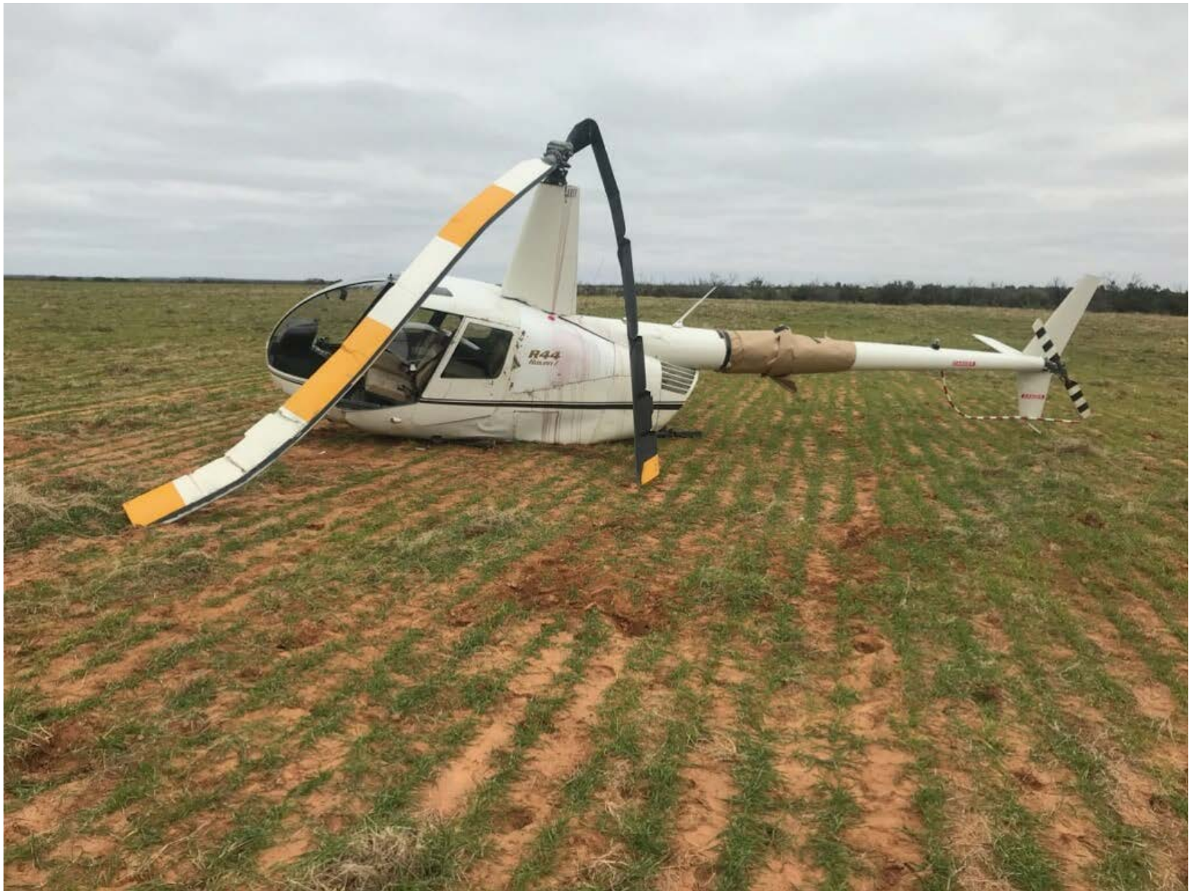
Photo 1 – View of damage to the main rotor system and fuselage (Courtesy of FAA)
