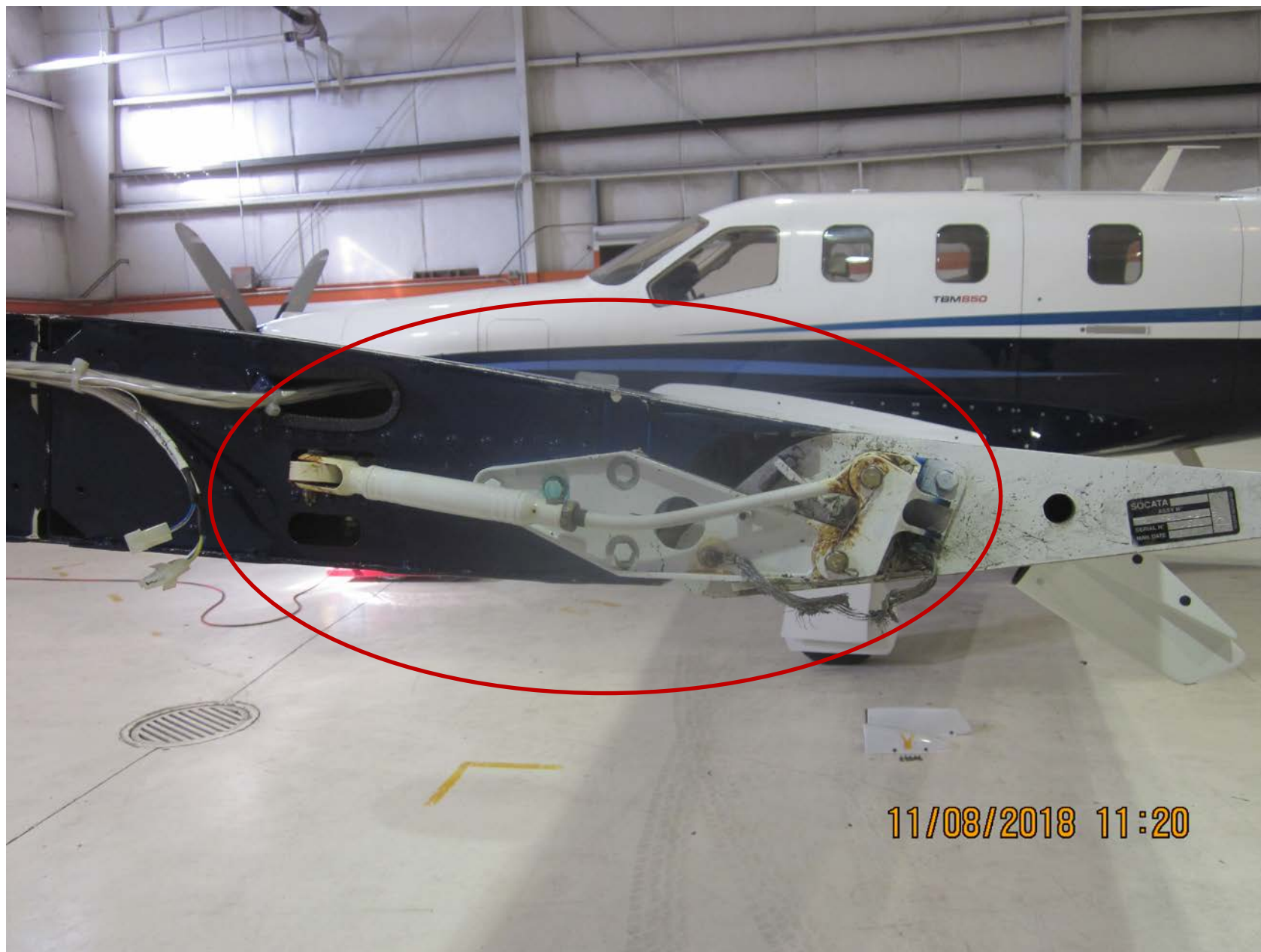
Photo 2 - View of bent left aileron control rod (photo courtesy of the FAA)
