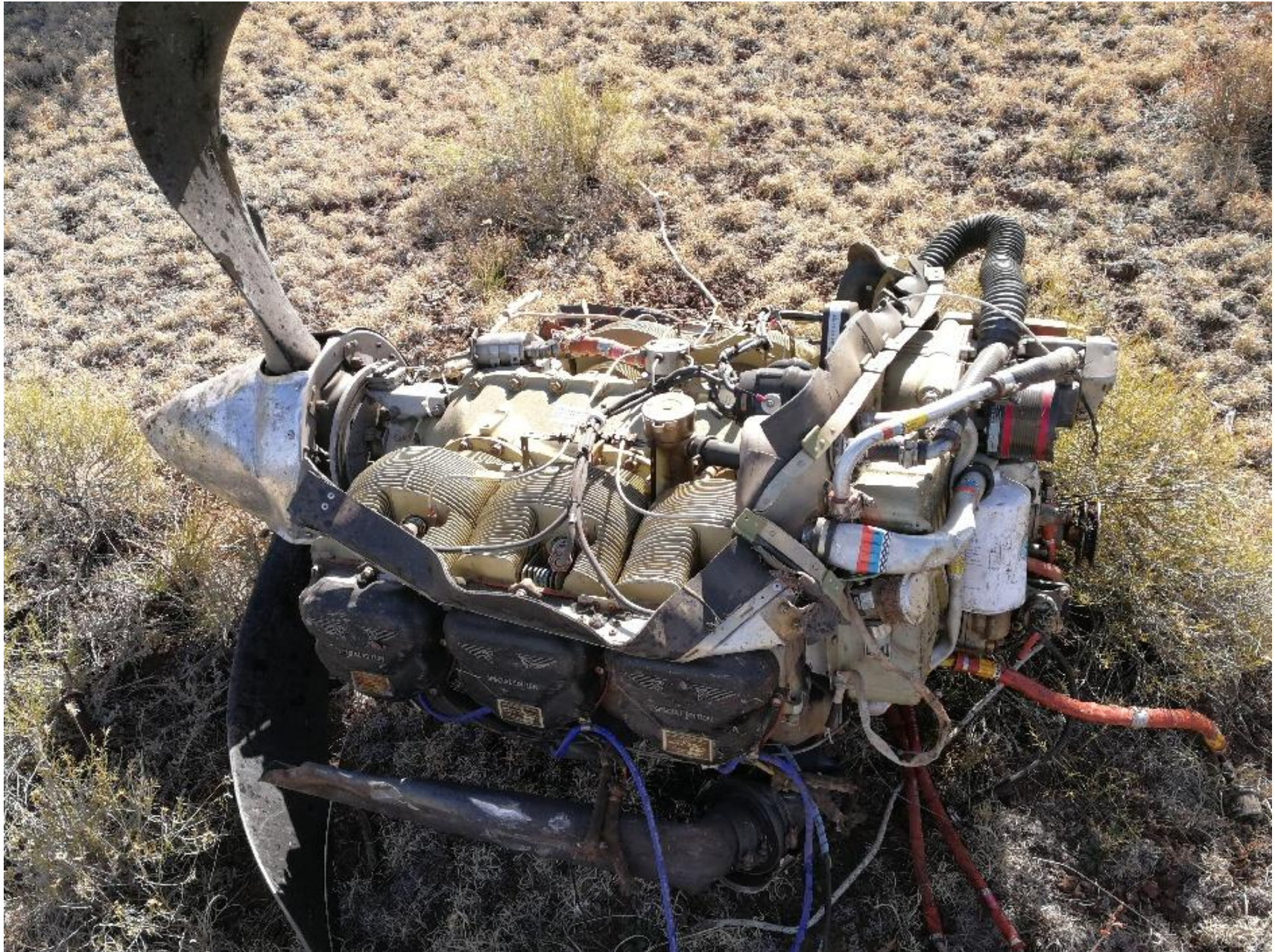
Photo 2 – View of separated engine (Photo courtesy unknown)
