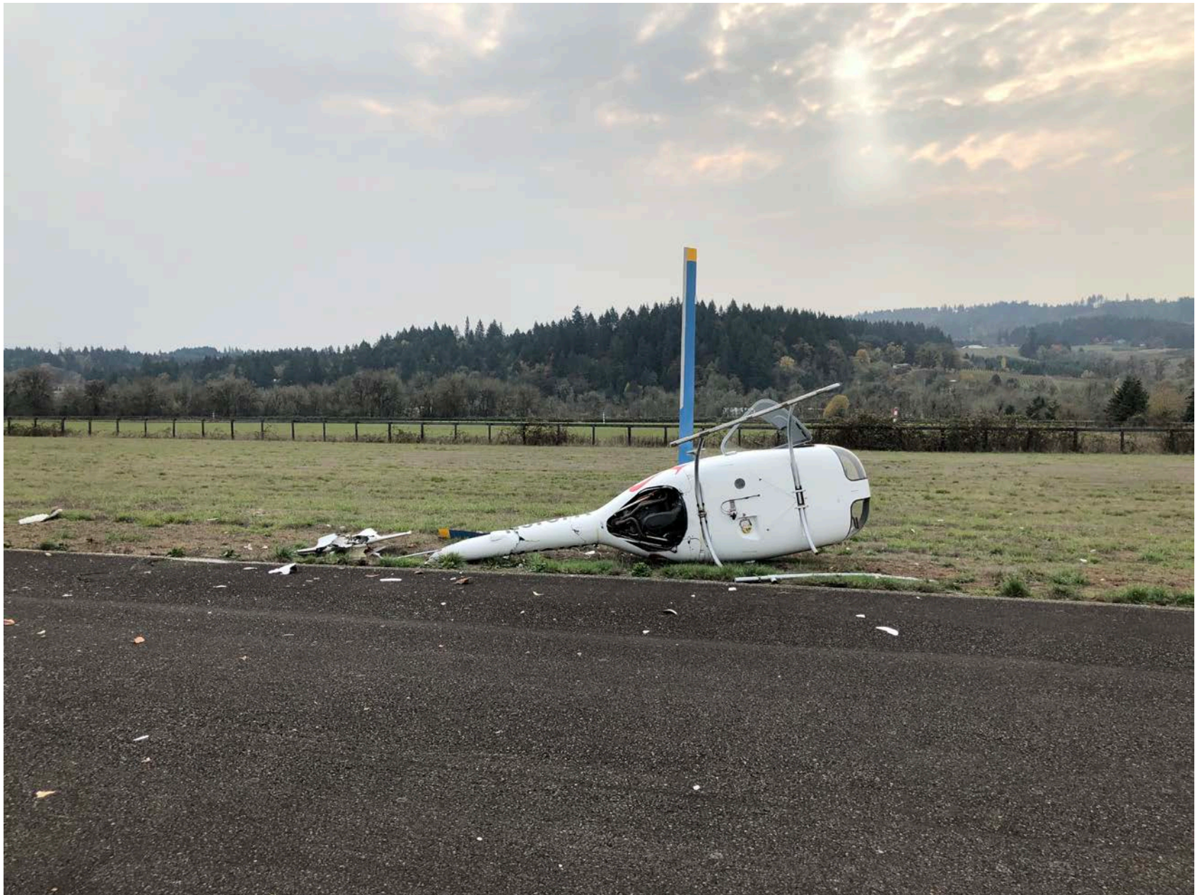
Photo 1 – View of damage to the tail rotor drive system (Courtesy of FAA)
