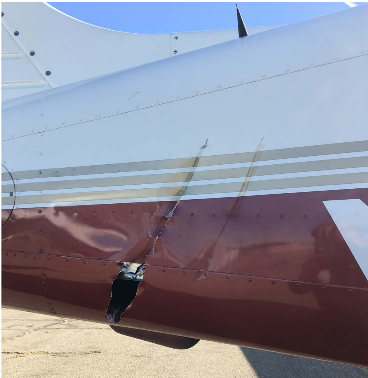
Photo 3 – View of damage to the right side empennage longeron (Courtesy of FAA)
