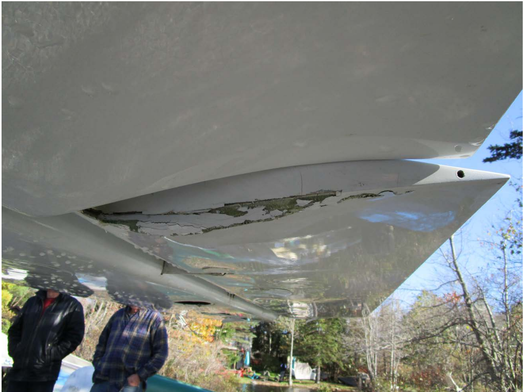
Photo 1 – View of damaged right aileron (courtesy of the FAA)
